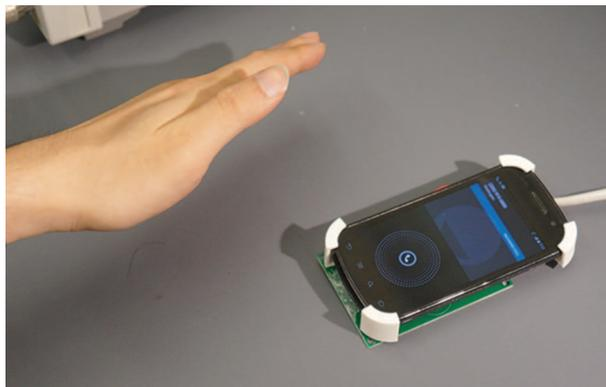
**[FIG1]** University of Washington researchers have created a new type of low-power wireless sensing technology that promises to allow users to “train” their smartphones to recognize and respond to specific hand gestures made near the phone. (Photo courtesy of the University of Washington.)
