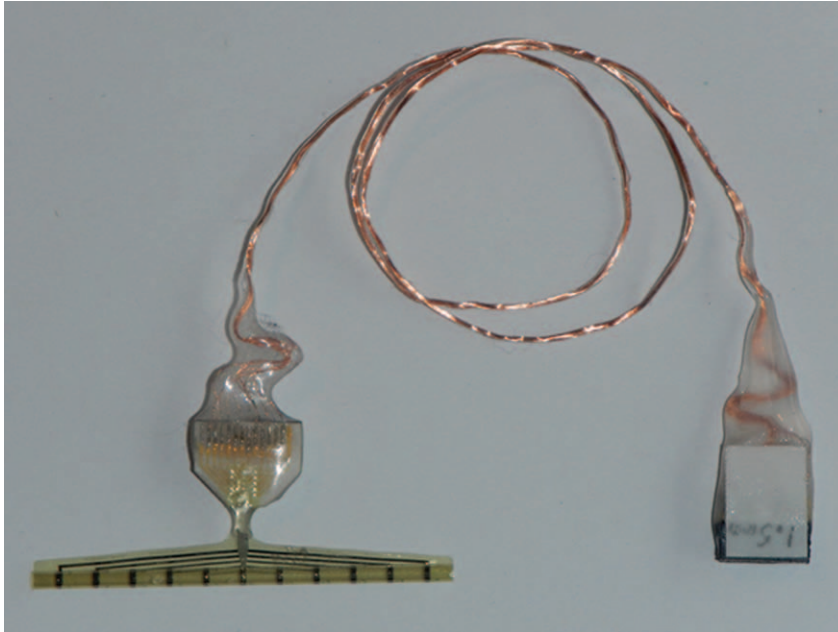
[FIG2] A multi-electrode nerve cuff used for velocity-selective recordings made by Martin Schuettler, a senior scientist at the University of Freiburg and chief technology officer of CorTek, a Freiburg, Germany-based developer of a neurotechnological platform for measuring and stimulating of brain activity. (Photo credit: Martin Schuettler.)
