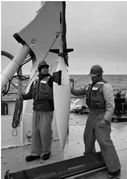
**Preparing to launch the University of Washington's Arctic Glider, designed to gather environmental data beneath the sea ice. (Photo courtesy University of Washington.)**
