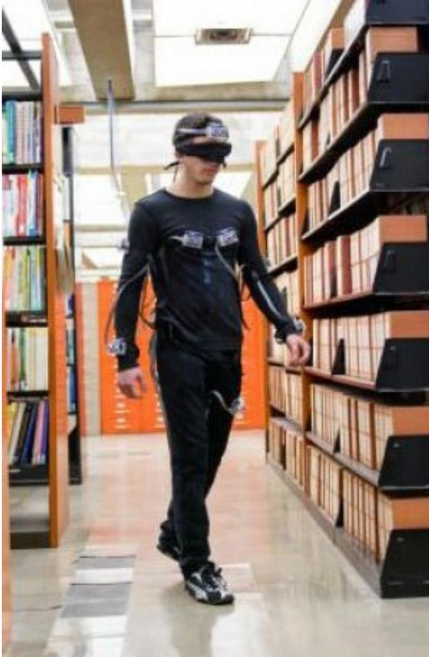
The system, which rapidly analyzes reflected pulses of sound or energy, mimics the way bats navigate their way across a terrain. Whenever a Spider-Sense module detects an approaching object, a servomotor worn by the user activates a pressure arm that pushes down on the wearer's body, functioning as a kind of electronic warning tap. The arm's pressure increases as the object gets closer.
