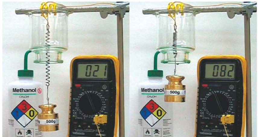
1. Ray Baughman, director of the University of Texas' NanoTech Institute, is developing materials that could be used for artificial muscles. For example, this NiTi spring has been coated with platinum nanoparticles (left). When it's heated to 70°C and above via a methanol/air mixture, the spring contracts and can lift a 500-g weight.
