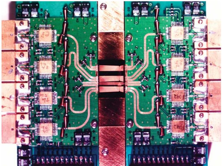
3. This optical arbitrary waveform generator chip (center) is packaged with high-speed driver electronics (left and right). Inphi Corp. provides the high-speed electronics, and Multiplex provides the semiconductor materials. (courtesy of S.J. Ben Yoo, Davis Branch Center for Information Technology Research in the Interest of Society, University of California, Davis)
