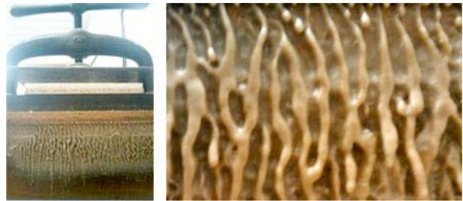
Figure 8: Traces of glue left on the side of the press
