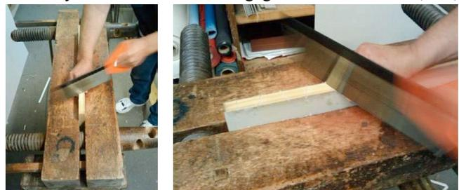
Figure 2: Sawing along edge of folded and nested pages that are held together in a wooden press.
