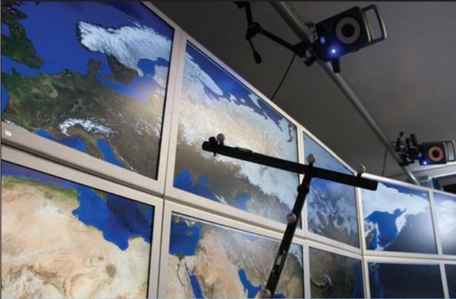
**Figure 4.** Multisurface interaction. Wall display in the WILD room consists of 32 off-the-shelf 30-inch monitors organized in an 8 × 4 grid.
