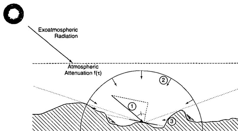
Figure 1. The three sources of solar radiation on a slope: (1) direct irradiance; (2) diffuse irradiance from the sky, where a portion of the overlying hemisphere may be blocked by nearby terrain; and (3) irradiance reflected off of nearby terrain. The solar illumination angle is  $i$  and atmospheric optical depth is  $\tau$ .
