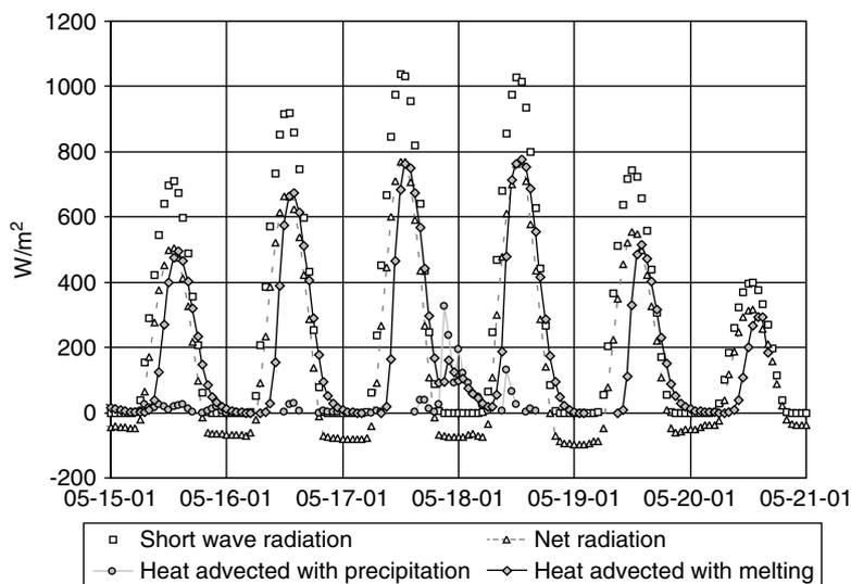
Figure 5. Simulated energy fluxes (a sample from the accumulation period) at the station, 15–25 May 2001
