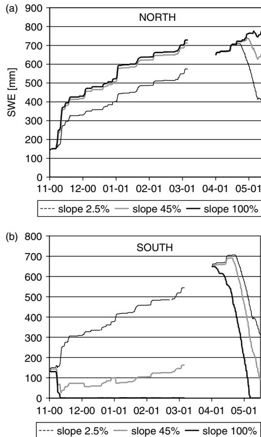
Figure 3. SWE evolution for sites with different slope and aspect; north and south aspects, 2.5, 45 and 100% slopes; separate simulations have been done for melting and accumulation seasons
