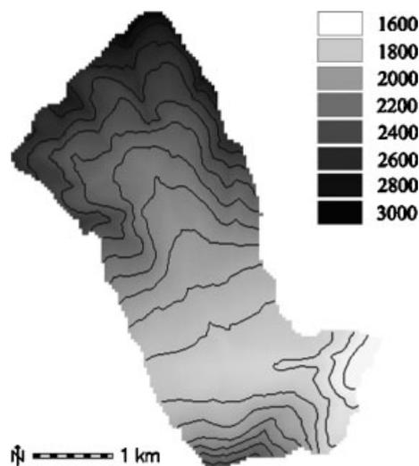
Figure 1. DEM of Rio Valbiolo catchment. Elevations are in metres
