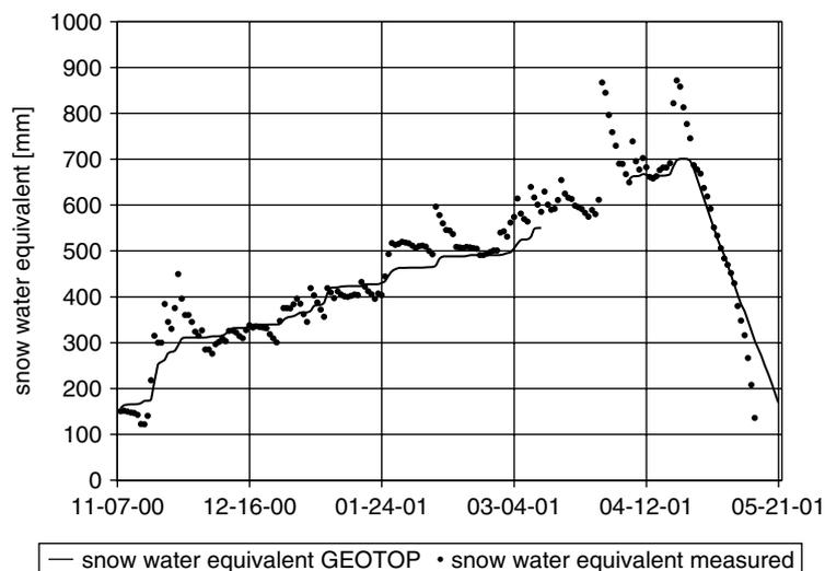
Figure 2. Simulated SWE at the meteorological station of Tonale pass (TN), compared with the measured SWE, 11 November 2000–21 May 2001
