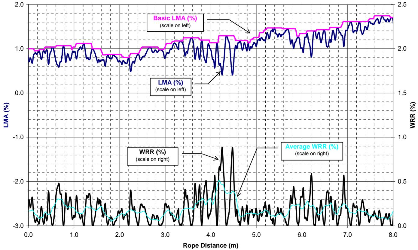
FIGURE 10. Rope 1, actual vs. estimated broken wire count
