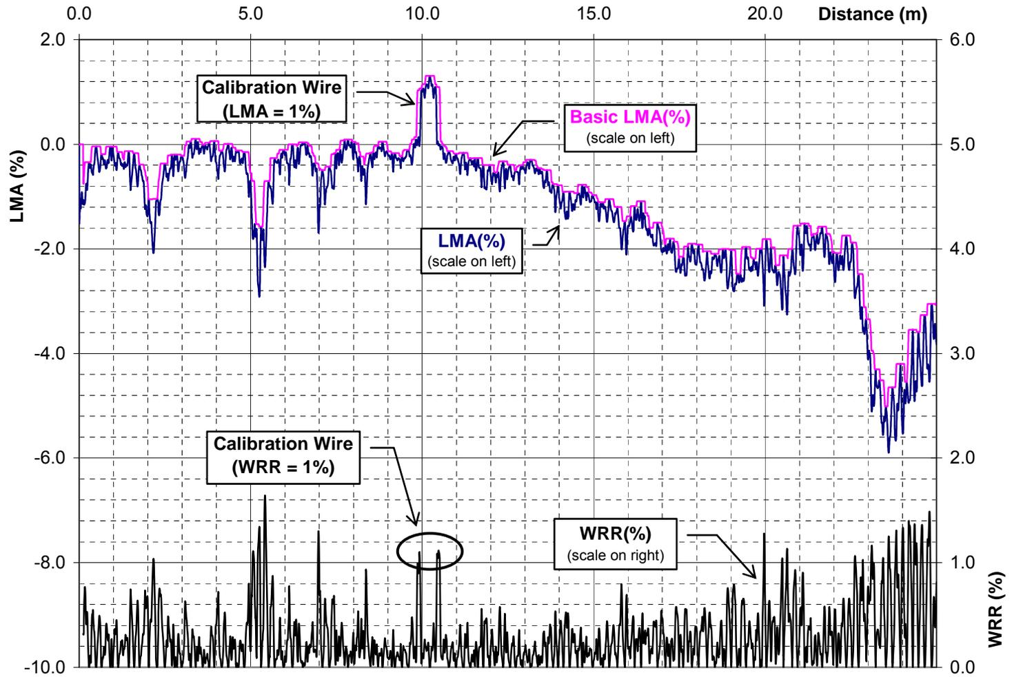
Rope 3 shows a maximum LMA of about 6%. This is less than the typical 10% LMA limit that is frequently used as a retirement condition. On the other hand, retirement based on a visual inspection after rope destranding was well justified.
