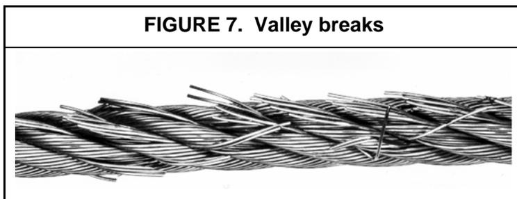
As the IWRC fails, the outer strands lose their radial support. This allows the wires of the outer strands to bear against each other tangentially. The resulting inter-strand nicking restricts the movement of the strands within the rope. Without this
