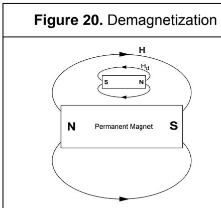
Consider the magnetic field  $H$  of a permanent magnet shown in Figure 20. If a ferromagnetic object is inserted into the field  $H$ , the object becomes magnetized and the field intensity,  $H$ , at the surface of the metal object is reduced from the value it was in the air.
