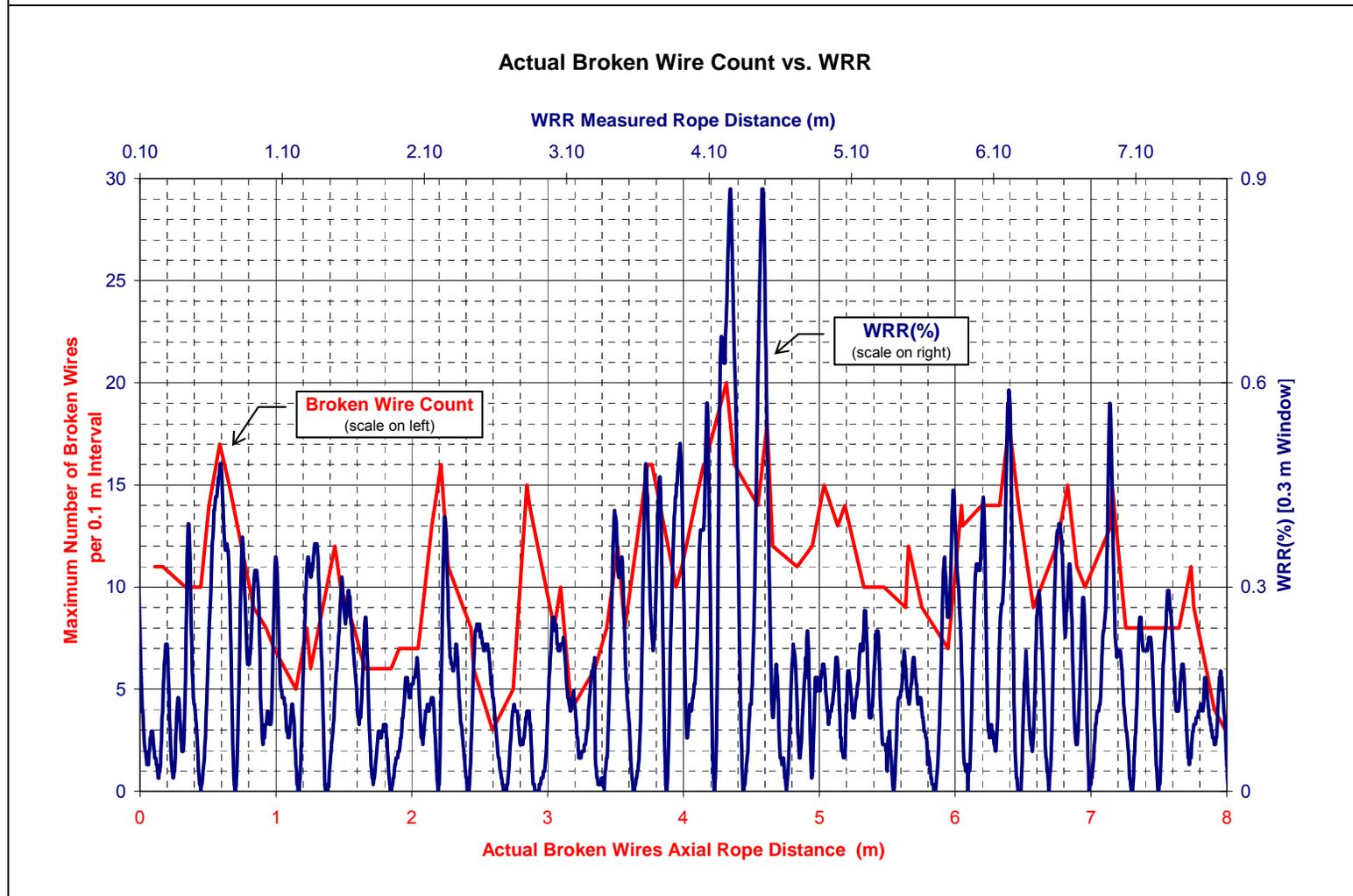
**FIGURE 12. Rope 1, comparison of broken wire count vs.  $WRR_p$
