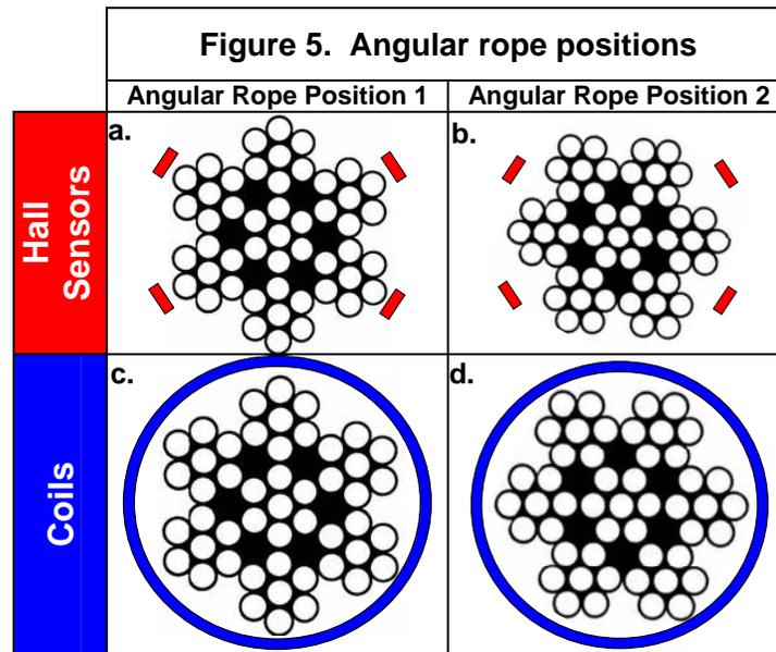
In contrast, coils circumscribe the rope. Therefore, coils-with-integrators sense the total combined magnetic flux in the rope, which – for new ropes – is independent of localized magnetic inhomogeneities inside the rope and circumferentially along the rope surface. In other words, the angular position of the rope inside the sensor head does not influence the signal. This situation is illustrated by Figures 5 c. and d.
