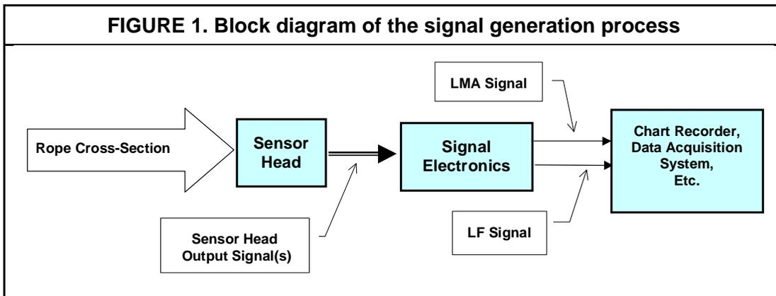
*Step changes of metallic cross-sectional area* – caused by missing or added wires, for example – have particular significance. Because of its simple geometry, a *step change of metallic cross-sectional area* can be called a *fundamental defect*. Accordingly, the corresponding LMA and LF signals, caused by a *fundamental defect*, can be called *fundamental LMA* or *LF signals*, respectively. The *fundamental signals* are collectively called an instrument's *step response*.
