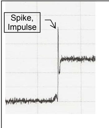
**FIGURE 7. Spike in the axial Hall sensor signal**
