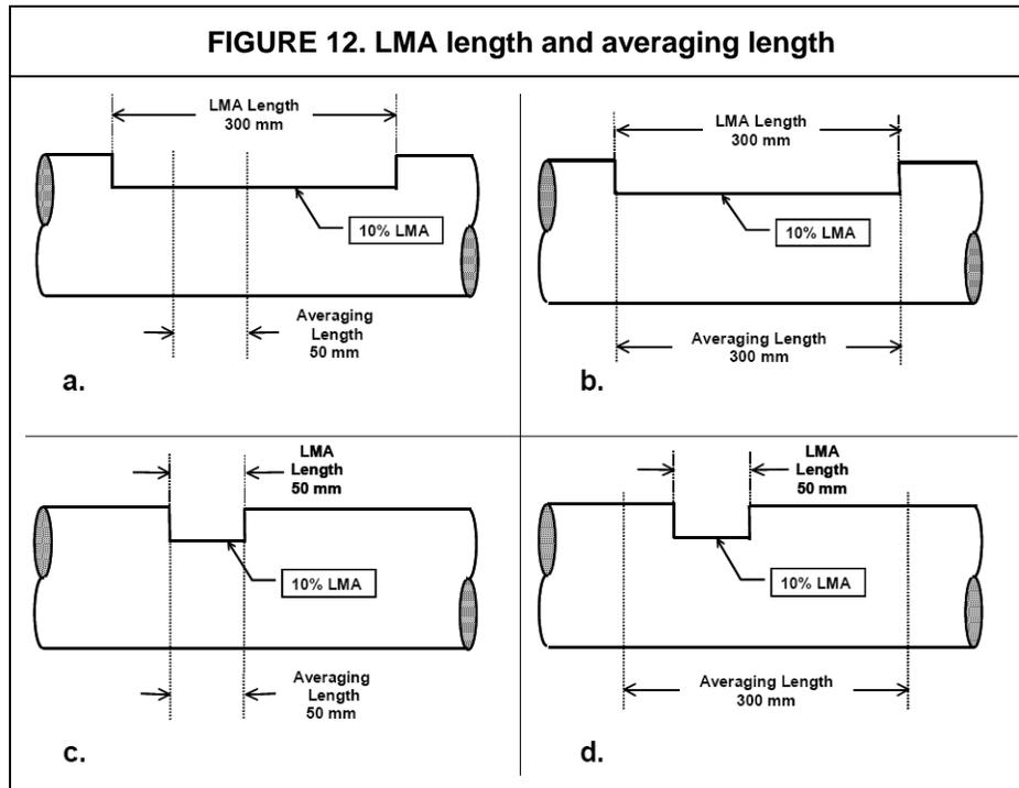
An analogy can illustrate the problems associated with long LMA averaging lengths: A chain is only as strong as its weakest link. Obviously, the strength of a chain is not determined by the average strength of some of its links. Similarly, the strength of a rope, which has lost metallic cross-section by corrosion and/or wear, is determined by the minimum local metallic cross-sectional area along the rope's length, and not by some average value of the rope cross-sectional area.
