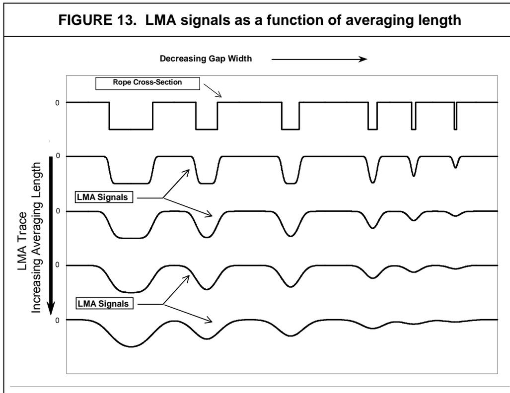
Because all wire rope testers have a *quantitative resolution* or *averaging length* that is greater than zero, an accurate measurement of LMA always requires minimum lengths of anomalies. As the above discussion shows and as illustrated by Figure 12, the concept of *quantitative resolution* or *averaging length* is important for specifying and comparing the performance of rope testers.
