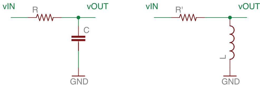
Figure 1: Basic  $RC$  and  $LR$  circuits. We use  $R = 1 \text{ k}\Omega$ ,  $C = 0.47 \mu\text{F}$ ,  $L = 33 \text{ mH}$ .
