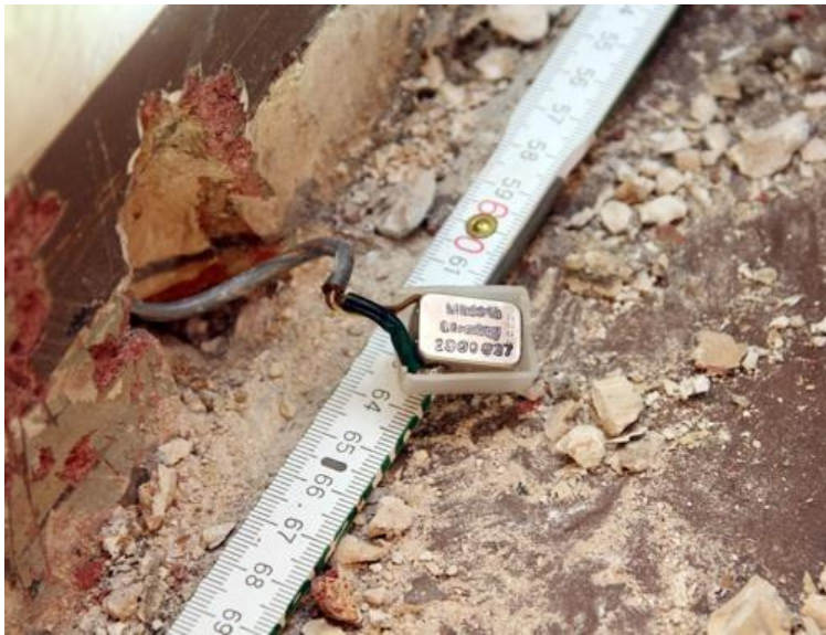
Figure 5: A hidden microphone in a cell wall in the former Stasi prison Bautzen II in Bautzen, Germany. Microphones in the jail cells listened to prisoners' conversations from behind the plaster, a few layers of paint. [Source: NY Post, Day in Photos: Dec. 14, 2011]
