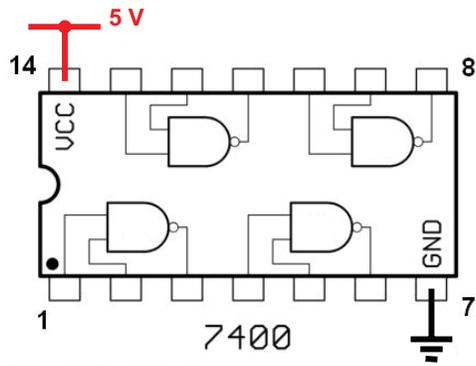
Figure 4: Pinout of the 74HC00, an integrated circuit version of the NAND gate.
