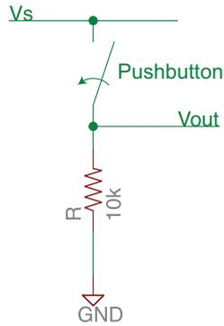
Figure 3: A simple push-button circuit.
