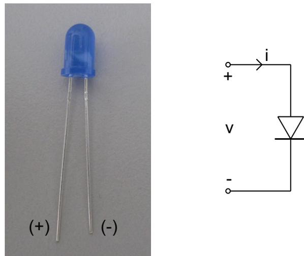
Figure 1: A photograph and schematic view of a light-emitting diode (LED). The lengths of the two leads indicate the positive and negative terminals of the diode.
