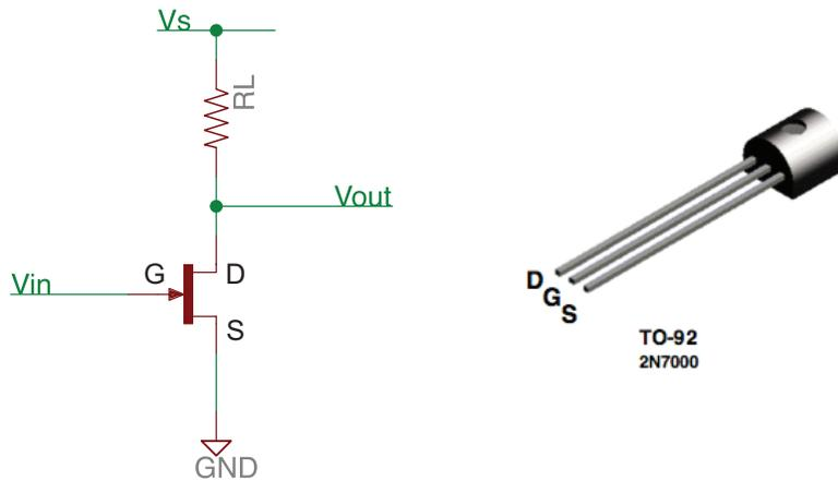
Figure 2: Basic MOSFET inverter circuit using the 2N-7000 transistor.
