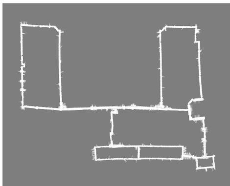
Fig. 6. MIT Killian Court dataset: occupancy grid map corresponding to the configuration estimated with the proposed technique. The size of the overall area shown in figure is approximatively  $250 \text{ m} \times 300 \text{ m}$ .
