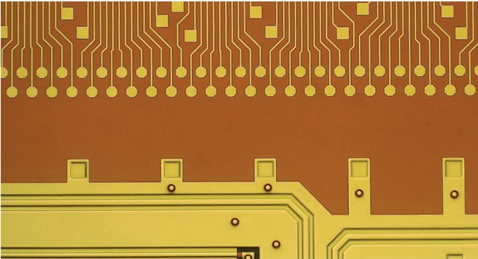
Metrigraphics' thin film process is a fundamental technology uniquely suited to the task of making miniature circuits with extremely small and uniform features that have extremely consistent electrical performance throughout.
