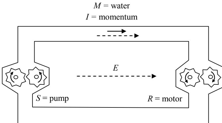
**Figure 3.** *Energy flow diagram, schematically describing a process where a pump transfers energy to a hydraulic motor, using for this the material carrier “water” and the immaterial carrier “momentum.”*
