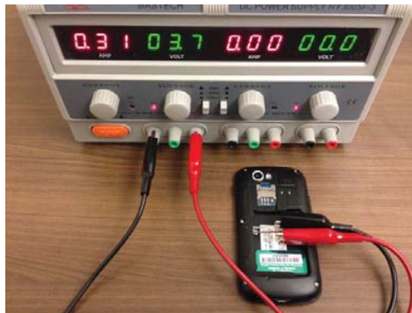
Fig. 1. Power metering system for energy measurement
