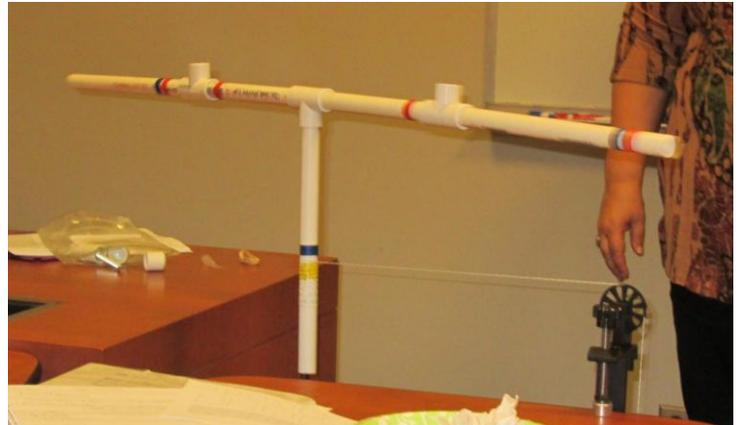
Martha asks the students to calculate the angular acceleration (they measure the acceleration of the falling weight) and the torque to calculate the amount of inertia. Pipes can be added vertically and/or horizontally to change the moment of inertia. Friction in the system produces some error but all the principles are clear to the students. Bolts can be placed into the pipes to increase mass. Martha also passed out a sheet showing how to use PVC pipes to build a white board stand (or easel).
