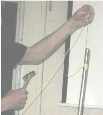
**Art Schmidt** (Northwestern University) used *Audioscope* software to show us the results of striking a steel rod in different places. First he struck the rod at one end (along its long axis), then in a direction perpendicular to the long axis. When the rod was struck end-on the fundamental frequency was about 2000 Hz; when it was struck across the long axis the fundamental was about 1000 Hz. When Art struck the rod at other places along its length we saw
