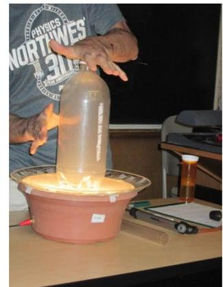
**John Papiewski** (NEIU) brought a Tesla coil he made and used it to light a CFL light bulb and a small fluorescent tube. John passed out a sheet with the circuit he used and various pieces of advice in case anyone wishes to try building one.
