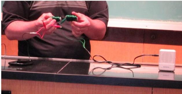
**John Lewis** brought a small audio amplifier and speaker from Radio Shack and any music playing device with headphones. He replaced the phones with an electromagnet made up of 30m of magnet wire wound on a large metal bolt. He made another identical electromagnet and used it on the input to the audio amp. When he turned on the music and brought the electromagnets near each other you could hear the music from the amp.
