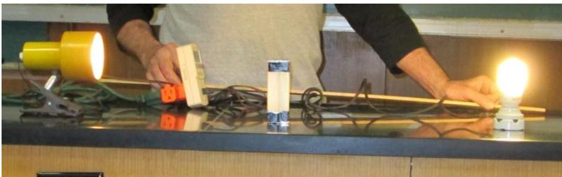
**Tom Senior** described a challenge between a compact fluorescent light bulb (CFL) and an incandescent bulb. They were both rated as equally bright. The power ratio was 75/13.5 watts. Tom took a wax sandwich comprised of two pieces of wax with a piece of aluminum foil between them. (This was a giveaway from
