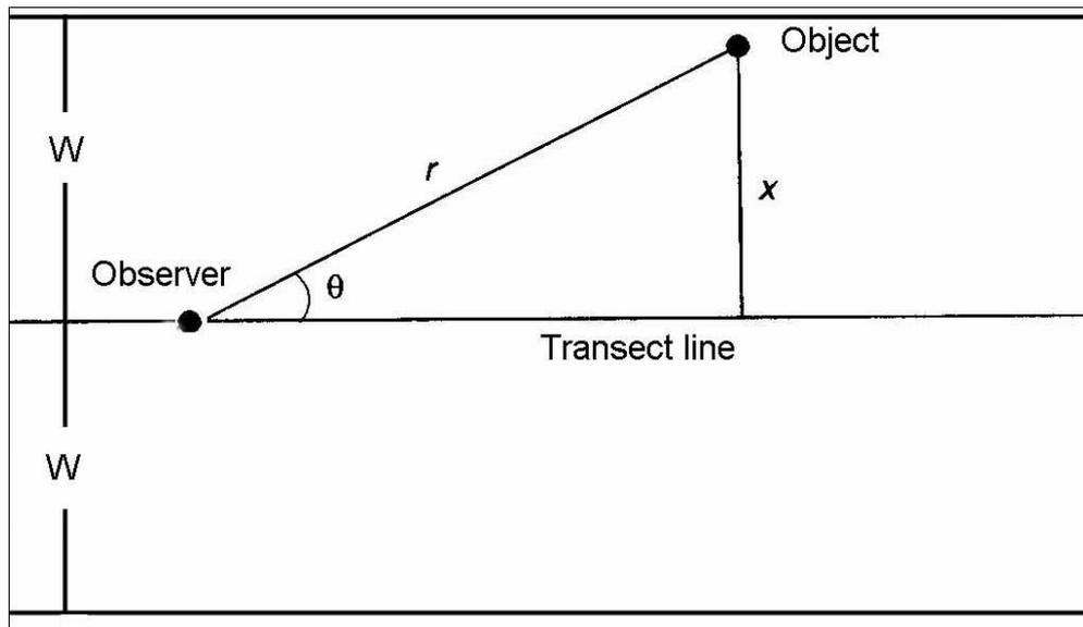
**Fig. 3:** Basic measurements that could be taken in line transect surveys. If  $r_i$  and  $\theta_i$  are taken,  $x_i$  is then found by simple trigonometry:  $x_i = r_i \cdot \sin(\theta_i)$ .
