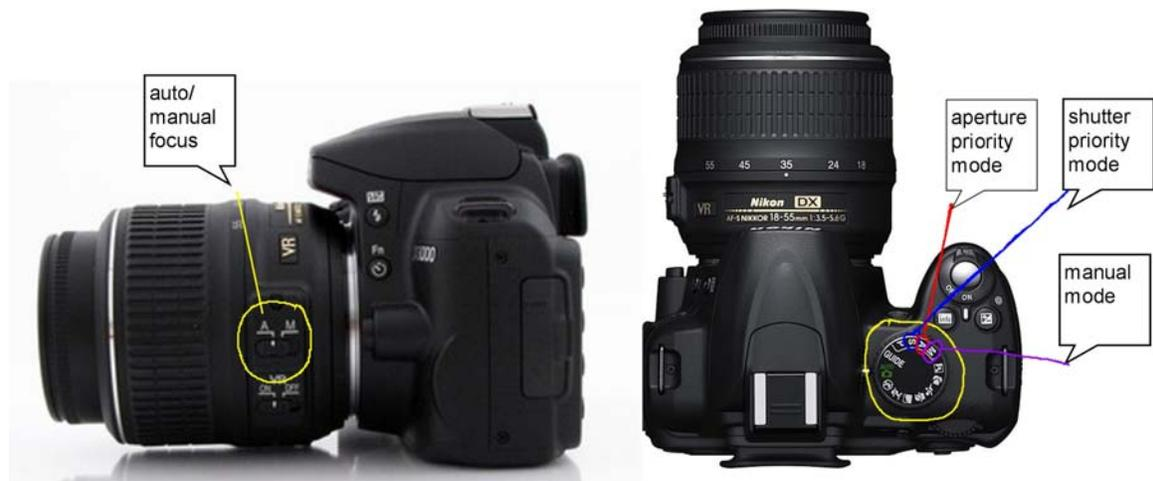
In the image above you see two images – on the left you see that I’ve circled the **manual focus** button on the lens (depending on your camera there may also be a switch on the body of the camera as well) this is **NOT** the place where you want to switch your camera to manual. When we are discussing shooting “in manual” we mean shooting in manual mode.
