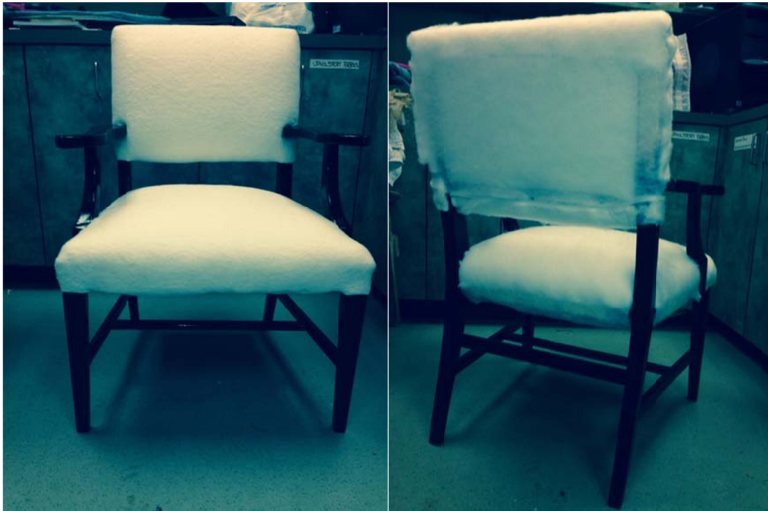
Figure 1.11: Left: Hepplewhite chair with muslin cover applied. Right: Rear view of the chair in the same stage.
