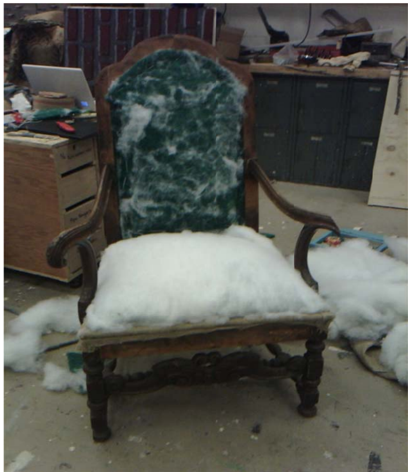
Figure 1.12: Armchair foundations with synthetic horsehair.
