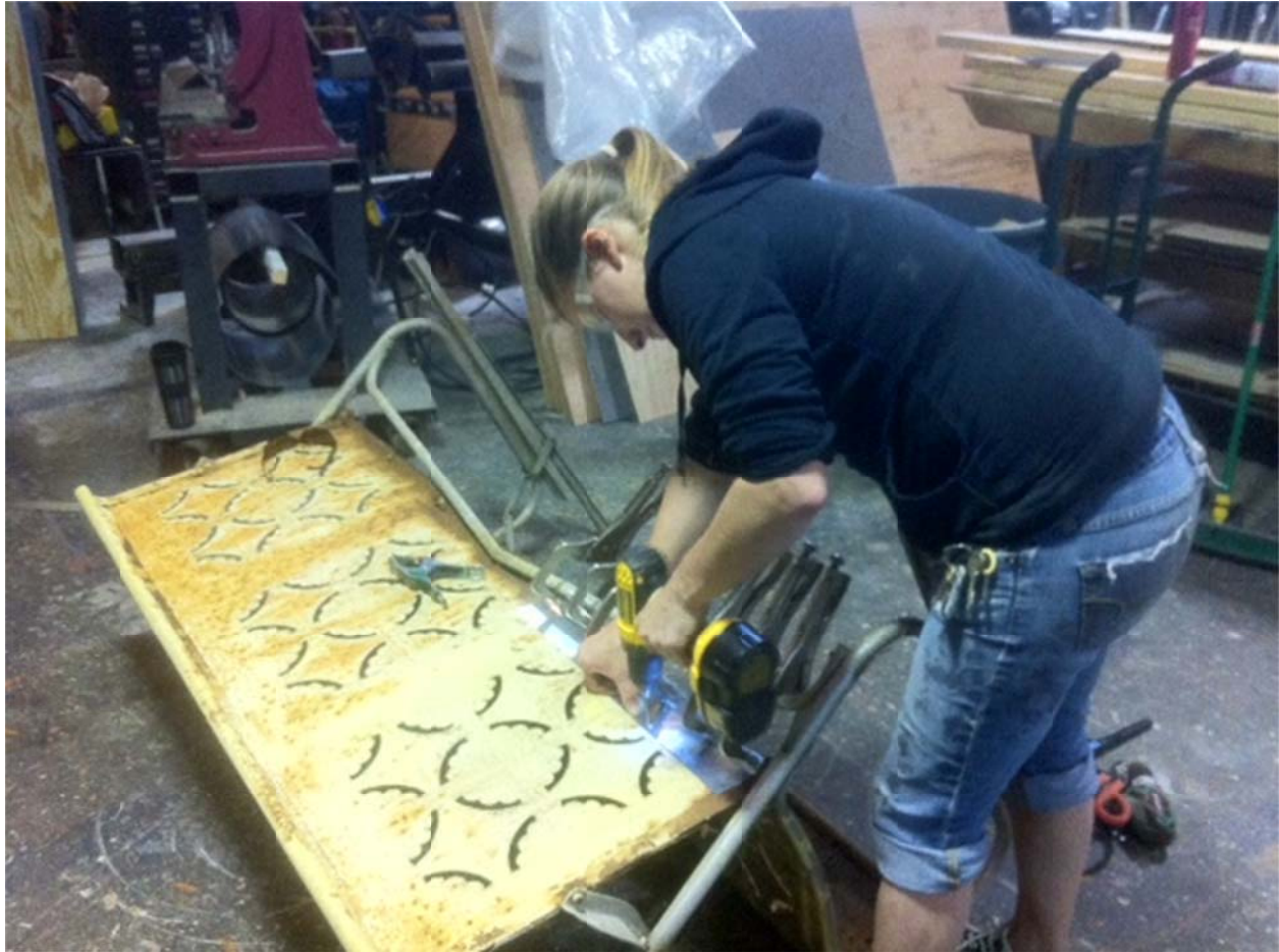
Figure 1.7: The author reinforces a glider using shaped aluminum pieces, vice grips, and steel rivets. She is seen here predrilling holes for the rivets. Photo by Chris Pyfrom.
