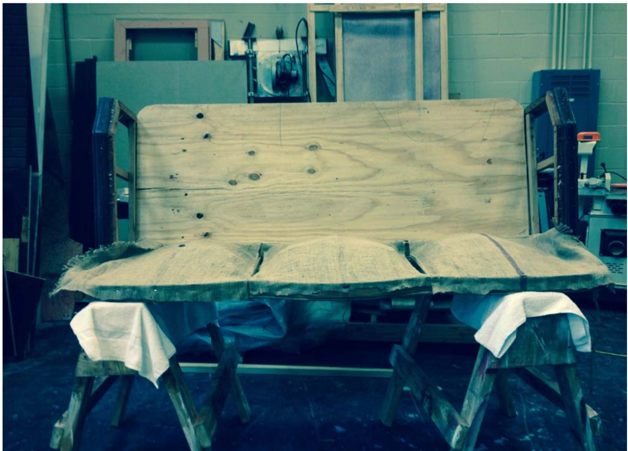
Figure 1.6: Couch frame with inserted plywood platform.
