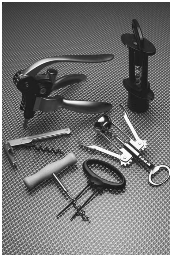
Types of corkscrews (clockwise from top left): single pump, screwpull, dual wing, Ah-so, T-pull, and pulltap.
