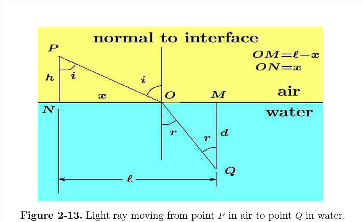
**Figure 2-13.** Light ray moving from point  $P$  in air to point  $Q$  in water.
