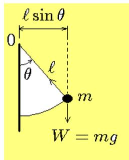
For the pendulum illustrated the forces about 0 are the weight of the mass and the radial force along the string. The radial force passes through the origin and so does not produce a moment about the origin. The moment of inertia of the mass  $m$  about 0 is given by  $I = m\ell^2$  and the torque about 0 is given by  $T = -(mg)(\ell \sin\theta)$  and consequently the equation of motion can be expressed  $T = -mgl \sin\theta = m\ell^2 \frac{d^2\theta}{dt^2}$
