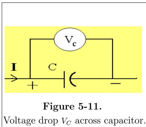
The **voltage drop  $V_C$  across a capacitance**, see figure 5-11, is proportional to the charge  $Q$  of the capacitance. The proportionality constant is denoted  $1/C$ . In symbols this is represented as
