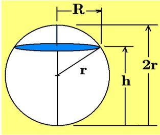
A spherical water tank has a radius of  $r = 12$  feet. Assume  $h = h(t)$  is the depth of the water in the spherical tank. The empty space above the water level inside the tank defines a spherical cap whose volume is given by  $V_{cap} = \frac{\pi}{3}(2r - h)^2(r + h)$
