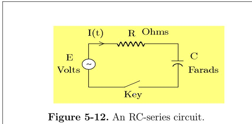
**Figure 5-12.** An RC-series circuit.
