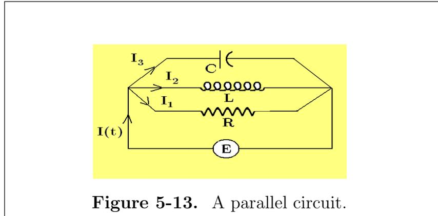
**Figure 5-13.** A parallel circuit.
