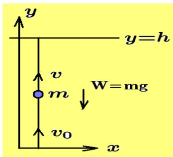
Consider a ball of mass  $m$  which is thrown vertically upward with an initial velocity  $v_0$ . Neglect air resistance so that the only force acting on the ball is the force due to gravity and construct a coordinate system with the origin placed at the point where the ball is released. Here the upward direction is taken as positive and by Newton's second law one can write
