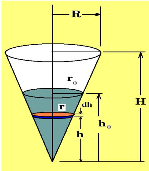
A right circular conical water tank, as illustrated has a top radius  $R$  and height  $H$ . Assume water is in the tank at a depth  $h_0$ . Let  $\omega = 62.5 \text{ lbs}/\text{ft}^3$  denote the density of water.
