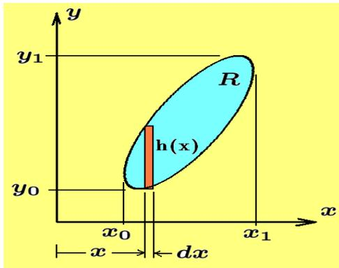
Pappus's<sup>25</sup> theorem states that if a region  $R$  is rotated about a line which does not pass through the region, then the volume of the solid of revolution equals the area of the region  $R$  multiplied by the distance traveled by the centroid of the region  $R$ . Assume the region  $R$  illustrated is rotated about the  $y$ -axis.
