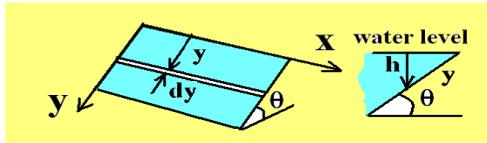
The face of a dam is a rectangular plate of width  $w$  and length  $\ell$ . The plate is inclined at an angle  $\theta$  so that the longer side is at the water level.
