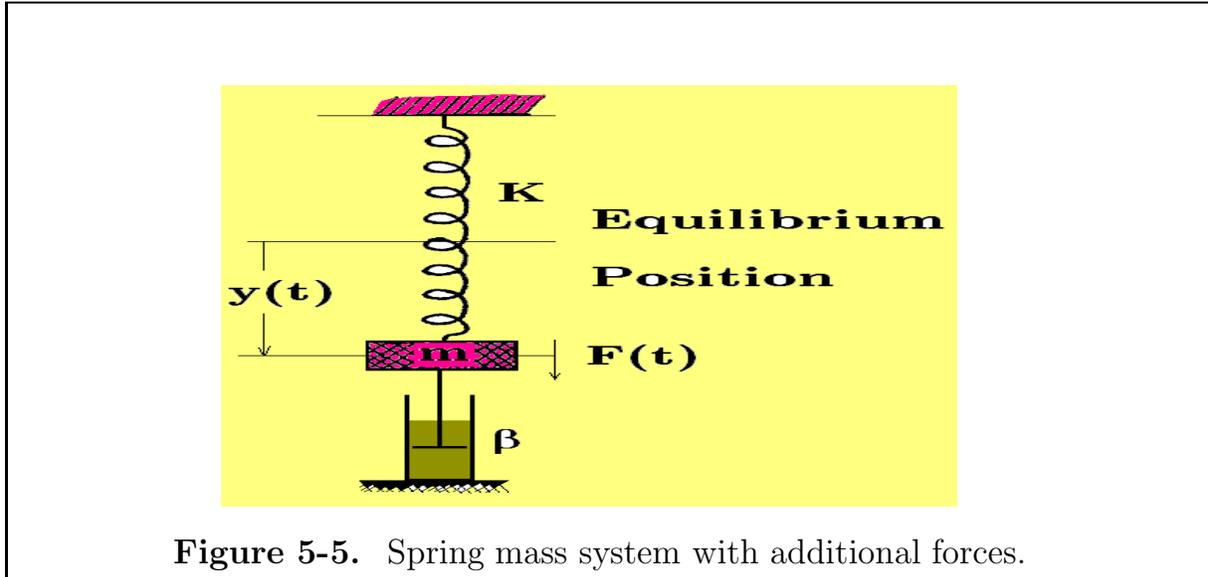
If there is a damping force  $F_D$  which opposes the motion of the mass and the **magnitude of the damping force is proportional to the velocity**<sup>12</sup>, then this can be represented by
