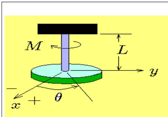
Figure 5-8. Torsional vibrations.
