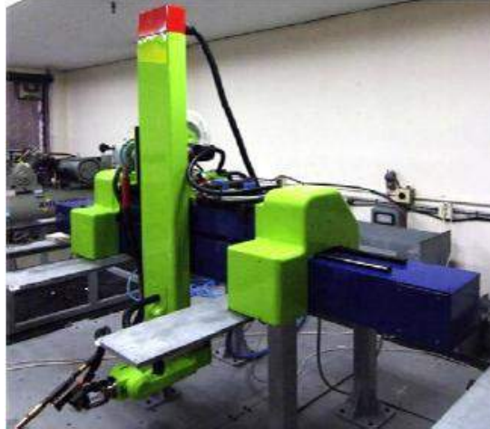
Figure 10. RRX4 Mobile Welding Robot
