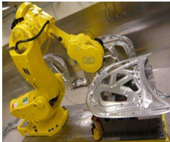
Figure 18. FSW robot welding automotive body parts at the Production Technology Centre
