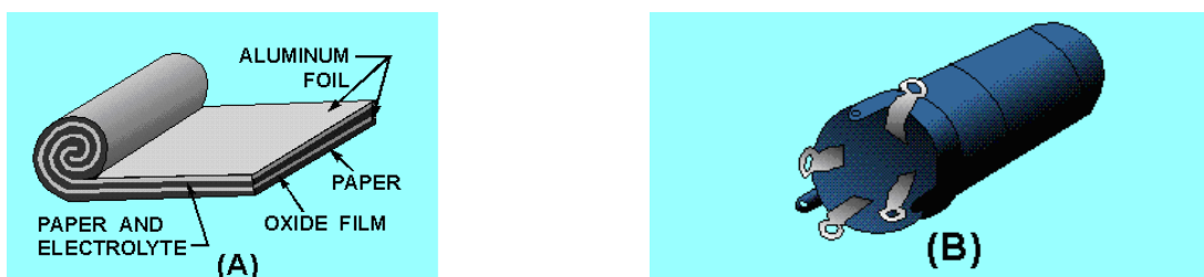
Figure 9-13. Construction (A) and common (B) view of an electrolytic capacitor
