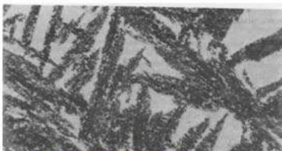
Bainite formed at 348°C
