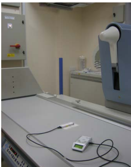
FIG. 22.3. Measurement of tube output using a calibrated solid state dosimeter which has lead backing to reduce backscatter. Note that the dosimeter and control unit are both shown in the photograph for demonstration purposes. In an actual situation, they would be further apart and the cable would not be coiled.
