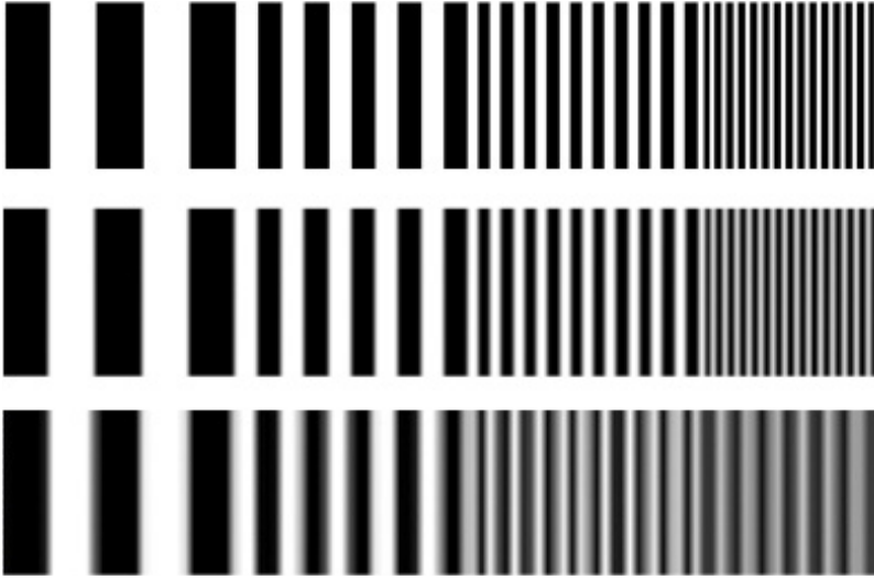
FIG. 7.7. Aliasing effect on the image of a bar pattern. Top: original. Centre: the pixel pitch is sufficiently small and all bar patterns are resolved correctly despite some blurring. Bottom: the pixel pitch is too large to resolve the finest bar pattern and aliasing occurs.
