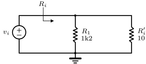
$$\therefore R_i = R_1 \parallel R'_i = 1\text{k}2 \parallel 10 \simeq 10 \Omega.$$
