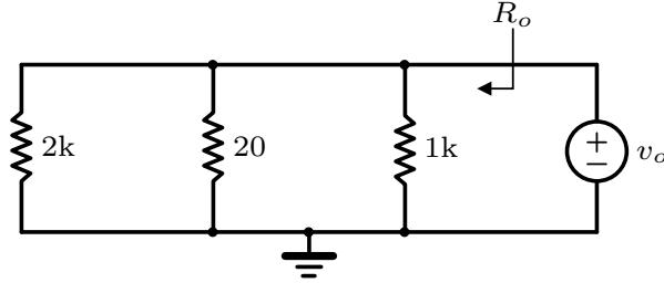
$$\therefore R_o = 2k \parallel 20 \parallel 1k = 1/(1/2k + 1/20 + 1/1k) \simeq 19.4 \Omega.$$
