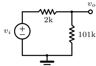
$$\therefore A_v = v_o/v_i = 101\text{k}/103\text{k} \simeq 0.98 \text{ V/V.}$$
