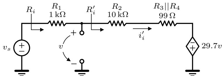
$$\therefore R'_i = \frac{v}{i'_i} = \frac{v}{(v+29.7v)/(10k+99)} \simeq 329\Omega \Rightarrow R_i = 1k + R'_i = 1329\Omega.$$
