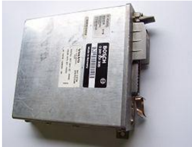
EDC control unit
