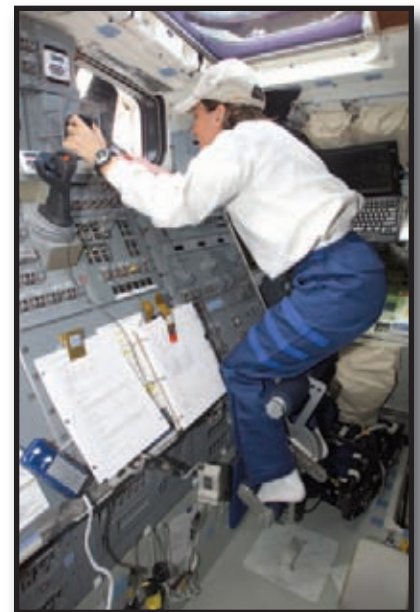
STS 109 Astronaut Nancy J. Currie, mission specialist, works the controls for the Remote Manipulator System (RMS) of Space Shuttle orbiter, Columbia
