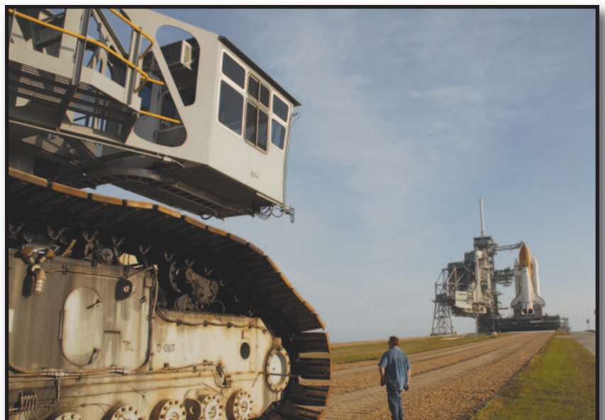
After delivering shuttle Discovery to the launch pad for the STS-124 mission, the crawler-transporter is moved to the foot of the pad
