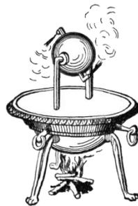
**Figura 6:** máquina de Heron. Knight's American Mechanical Dictionary, 1876. Wikipedia
