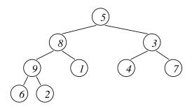
Then the rearrangement algorithm starts by bubbling down a[n/2] = a[4] = 9, which turns out not to be necessary, so the array remains the same. Next a[3] = 3 is bubbled down, swapping with a[7] = 7, giving:
