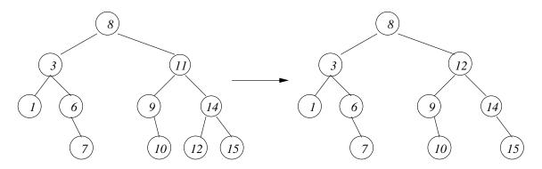
Figure 7.1: Example of node deletion in a binary search tree.
