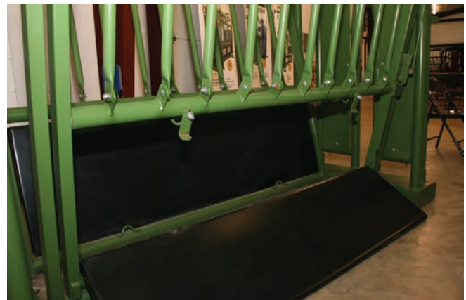
FIGURE 11-3. Lower panels can be removed to access the cattle's feet and legs.
