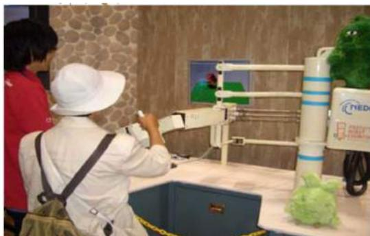
Fig. 6. Rehabilitation system "Robotherapist".
