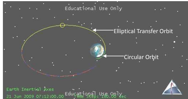
Figure 5. Satellites in the transfer elliptical orbit.
