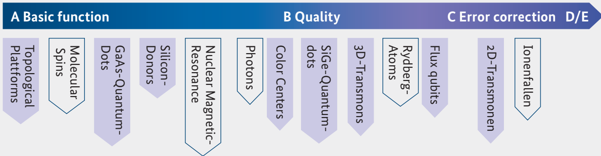
Figure: Classification of different platforms in the layer model. Source: BSI study "Status of quantum computer development".
