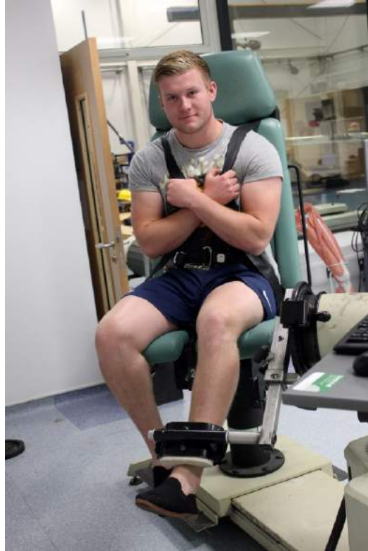
Figure 4. 2 The Cybex dynamometer and participant position.
