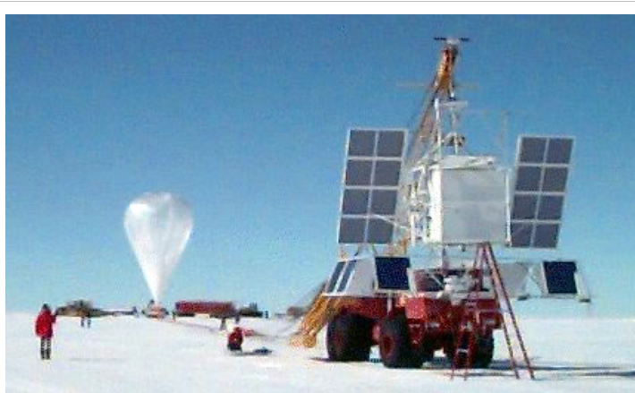
HIREGS attached to launch vehicle while balloon is inflated (1993)
