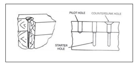
Figure 2-8. Sinking a wood screw properly
