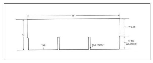
Figure 7-23. Square-butt asphalt strip shingle
