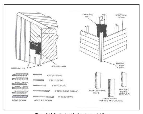
Figure 6-43. Vertical and horizontal wood siding
