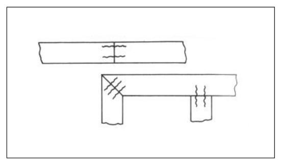
Figure 2-17. Proper use of corrugated fasteners
