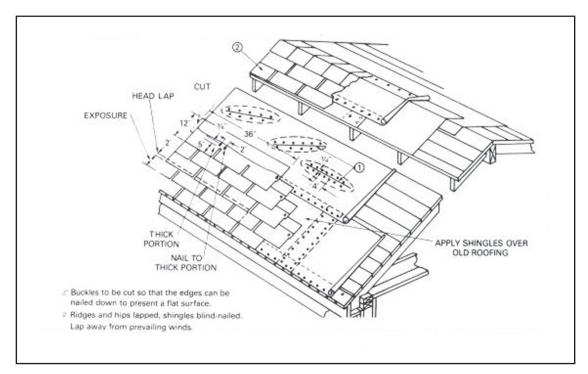
Figure 7-30. Roof replacement
