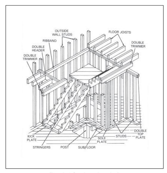
Figure 6-52. Complete stairway detail
