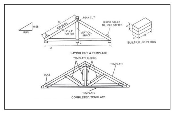
Figure 7-19. Laying out and assembling with a template
