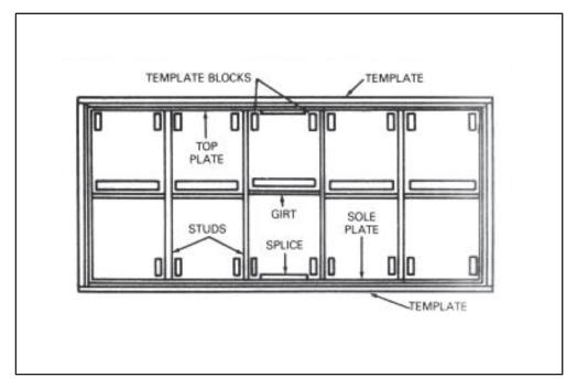
Figure 2-1. Template for framing walls
