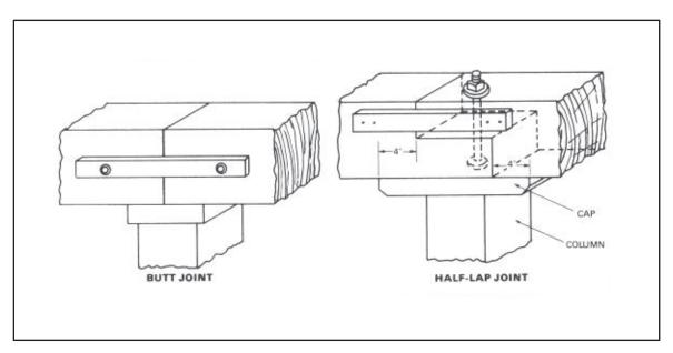
Figure 6-14. Butt and half-lap joints
