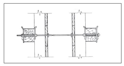
Figure 5-9. Tie rod and spreader combination
