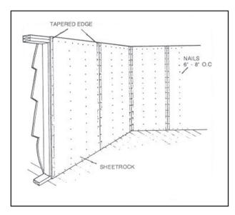
Figure 9-3. Sheetrock applied vertically
