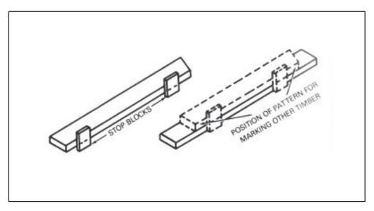
Figure 2-2. Marking a pattern
