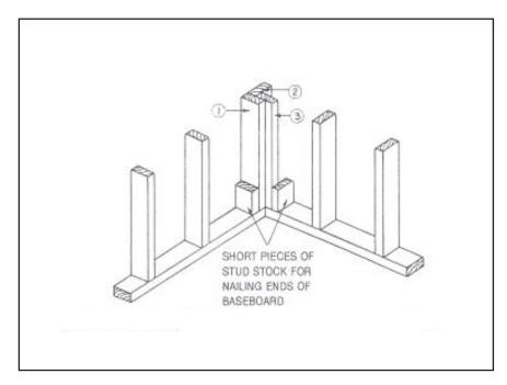
Figure 6-30. Corner-post construction using ordinary 2 x 4 studs
