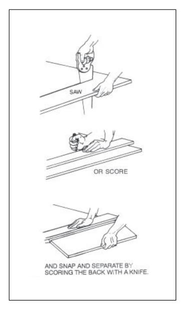
Figure 9-5. Cutting sheetrock
