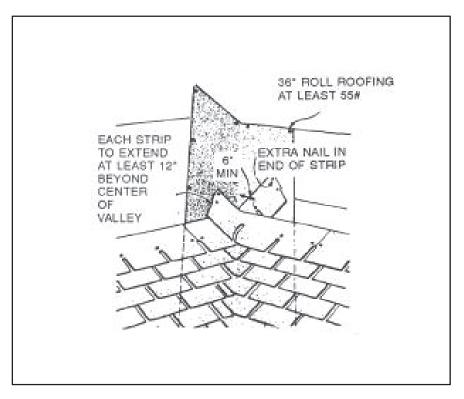
Figure 7-32. Closed-valley flashing using woven strip shingles
