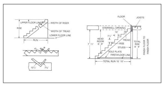
Figure 6-51. Step construction
