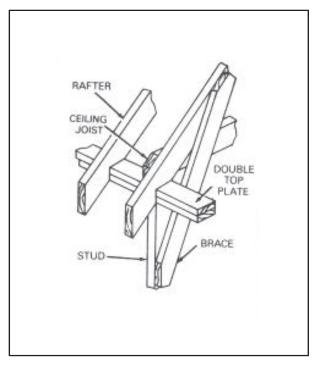
Figure 6-46. One method of bracing attic plate
