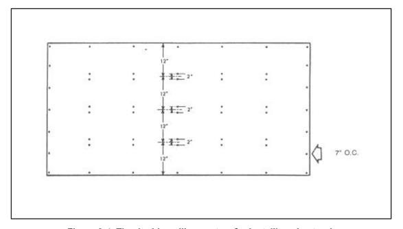
Figure 9-4. The double-nailing system for installing sheetrock
