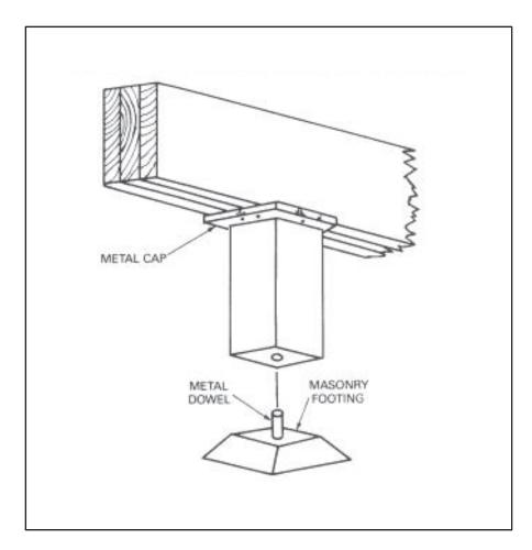
Figure 6-15. Use of metal cap and masonry footing
