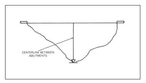
Figure 10-12. Determining trestle-bent height
