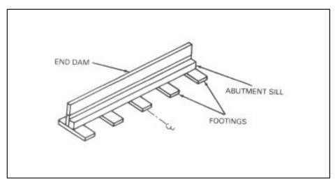
Figure 10-2. Timber sill abutment
