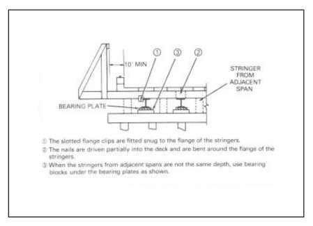
Figure 10-15. Open laminated deck, sectional view
