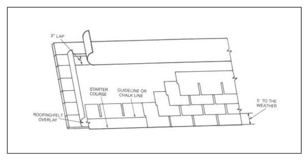
Figure 7-24. Laying an asphalt-shingle roof
