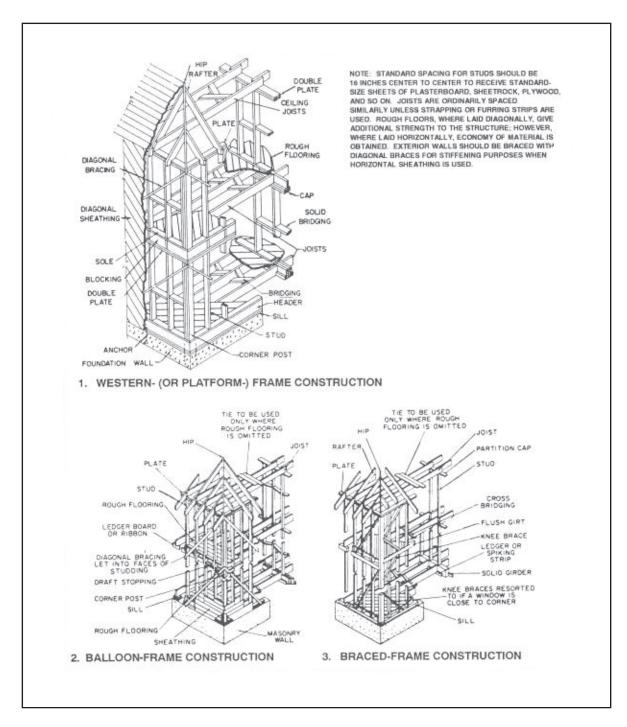
Figure 6-1. Framing for light structures
