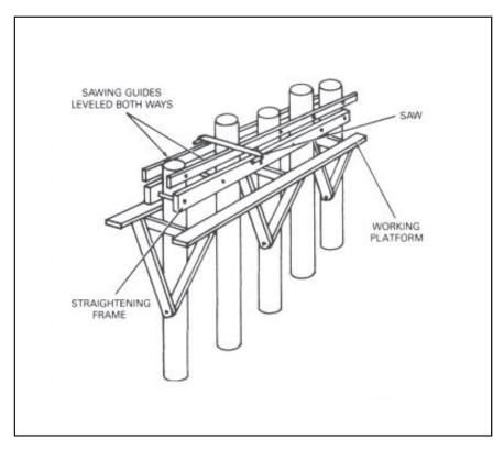
Figure 11-7. Cutting piles
