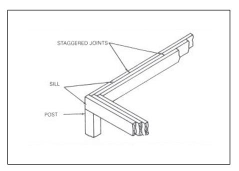
Figure 6-9. Corner joint of a built-up sill
