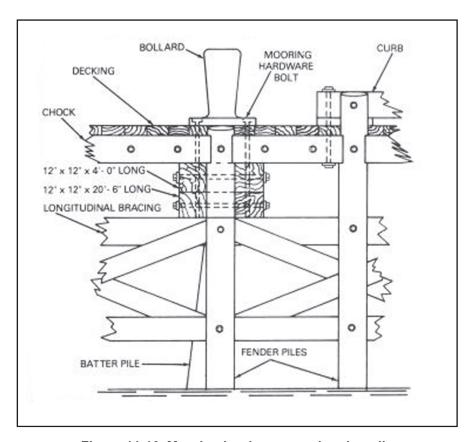
Figure 11-16. Mooring hardware over bearing pile
