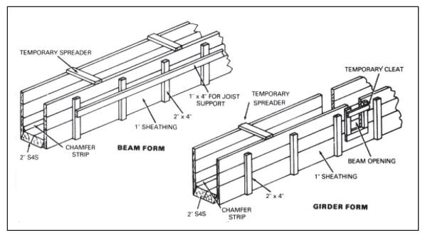
Figure 5-12. Beam and girder forms
