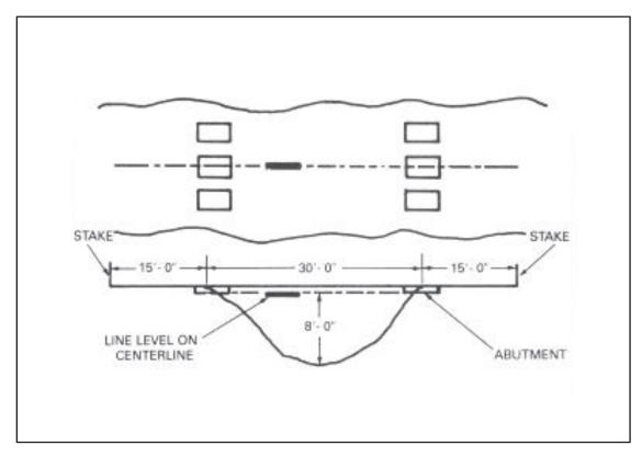
Figure 10-9. Laying out a centerline
