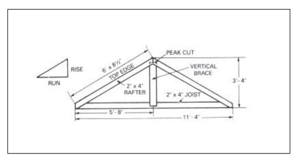
Figure 7-15. Truss layout
