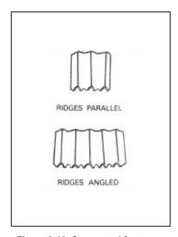
Figure 2-16. Corrugated fasteners
