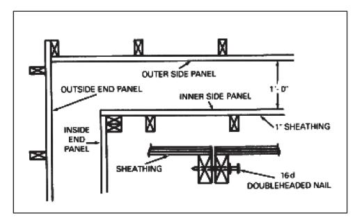
Figure 5-6. Constructing wall panels
