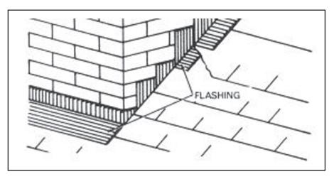
Figure 7-29. Vertical wall flashing
