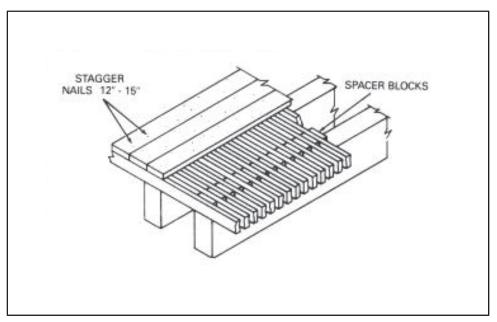
Figure 10-16. Open laminated deck
