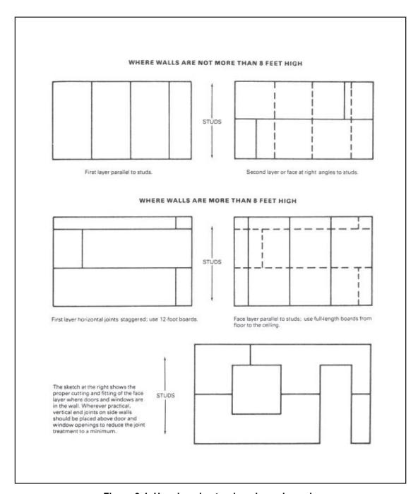
Figure 9-1. Hanging sheetrock and wood panels
