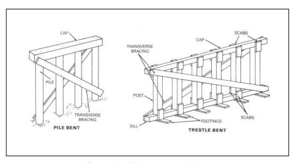
Figure 10-4. Pile bent and trestle bent
