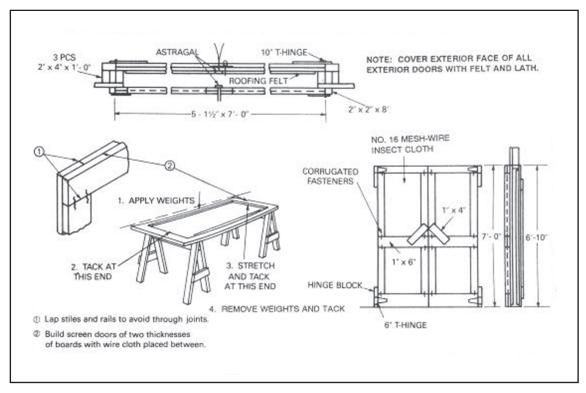
Figure 8-16. Door screen construction
