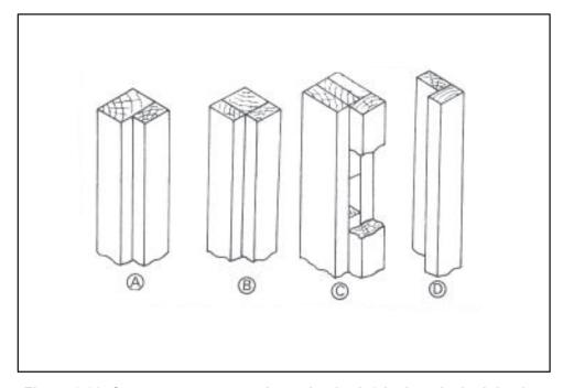
Figure 6-32. Corner-post construction using both 2-inch and 4-inch lumber
