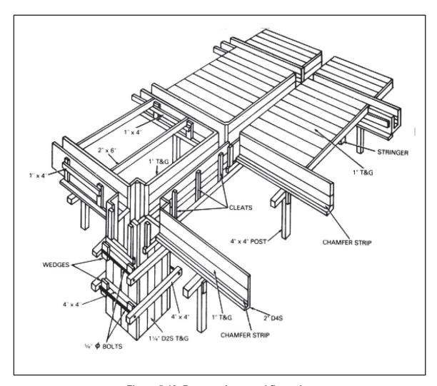
Figure 5-13. Beam, column and floor plan
