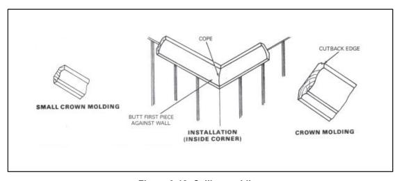
Figure 9-12. Ceiling molding
