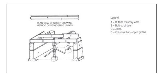
Figure 6-10. Built-up girder details
