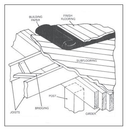
Figure 6-18. Floor joists
