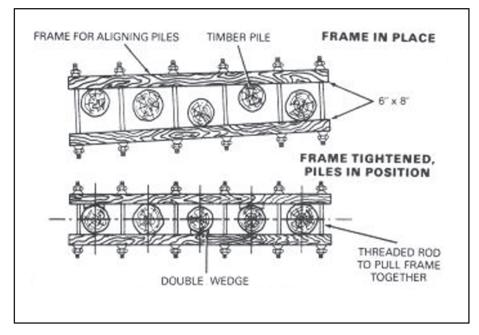
Figure 11-5. Realigning with a frame
