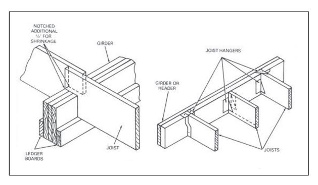
Figure 6-11. Joist-to-girder attachment
