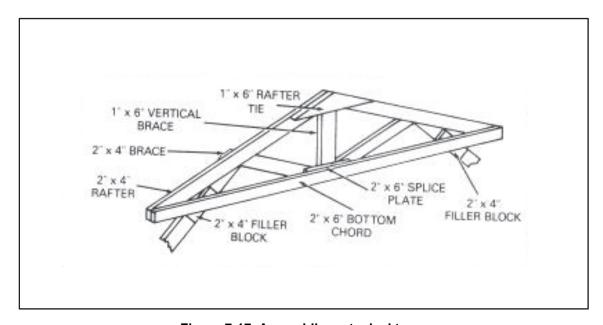
Figure 7-17. Assembling a typical truss
