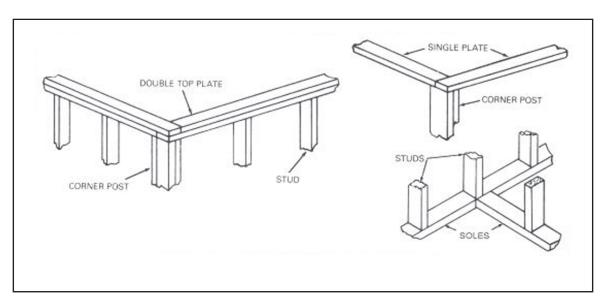
Figure 6-36. Top-plate and sole-plate construction
