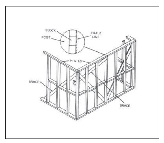
Figure 6-39. Straightening a wall
