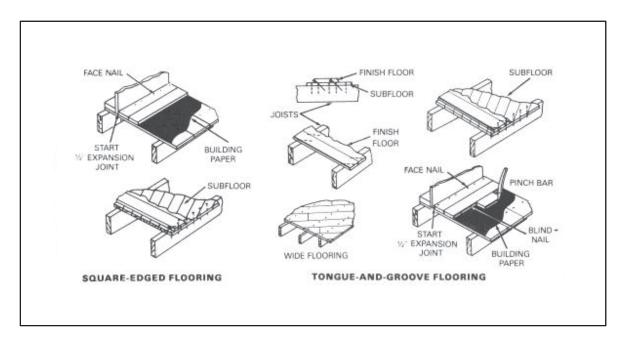
Figure 6-27. Square-edged and tongue-and-groove finish flooring
