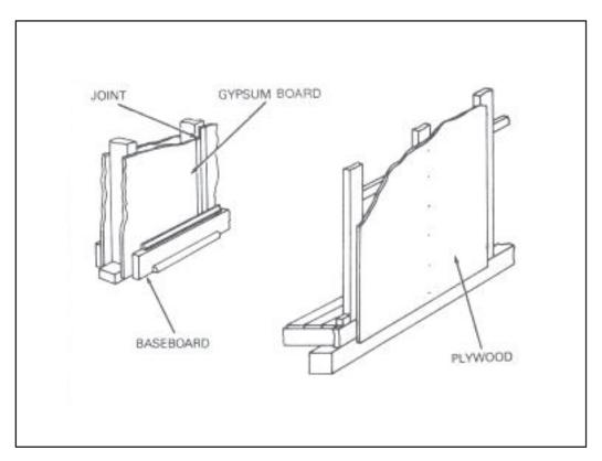
Figure 6-42. Gypsum and plywood sheathing
