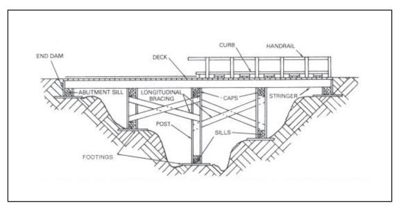
Figure 10-1. Nonstandard fixed highway bridge
