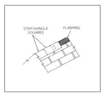
Figure 7-26. Hip or ridge flashing
