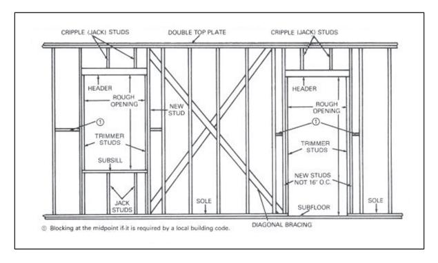
Figure 6-28. Typical wall-frame details
