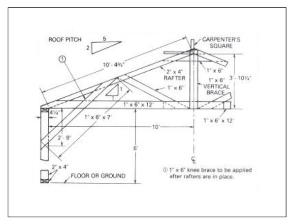
Figure 7-18. Truss- or rafter-support detail
