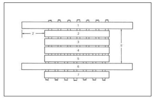
Figure 10-18. Extended deck for handrail support
