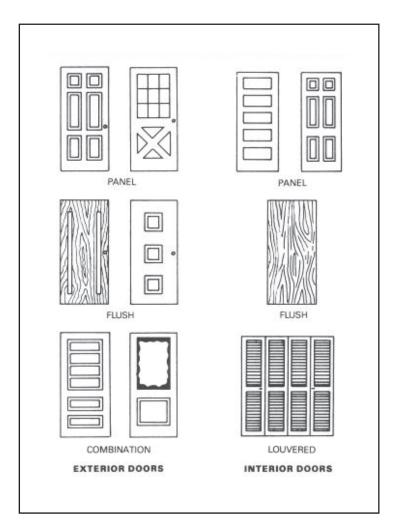
Figure 8-2. Mill-built doors
