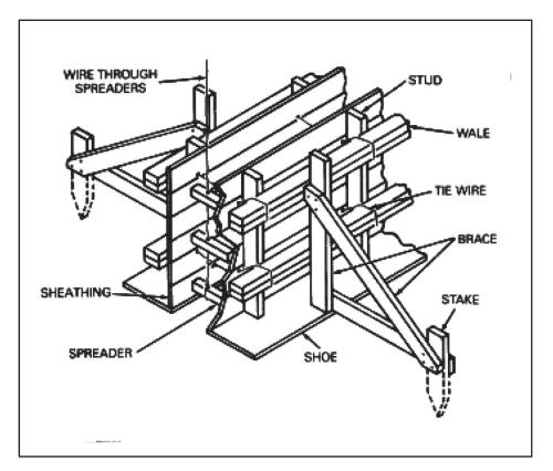
Figure 5-5. Concrete wall form
