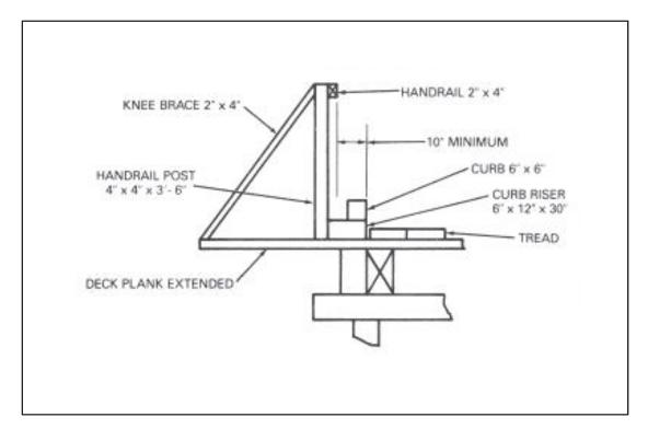
Figure 10-20. Standard curb and handrail
