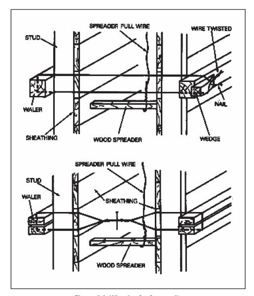
Figure 5-8. Wire ties for form walls
