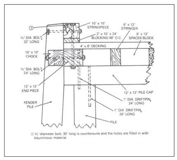
Figure 11-11. Wharf-edge cross-section of a timber-pile wharf
