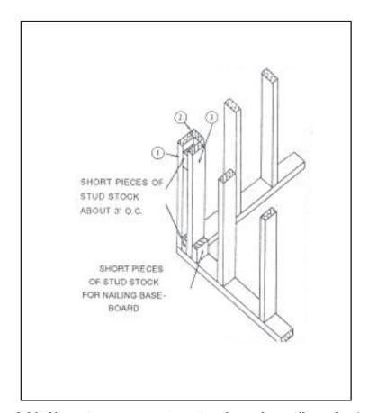
Figure 6-31. Alternate corner-post construction using ordinary 2 x 4 studs
