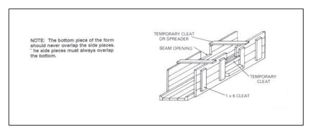
Figure 6-17. Girder and beam form
