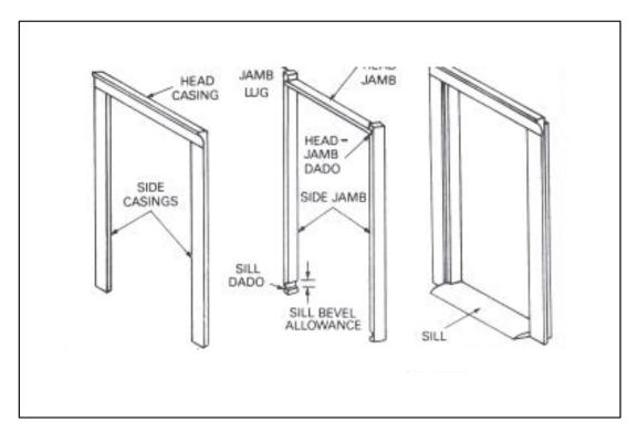
Figure 8-3. Principal parts of a door frame
