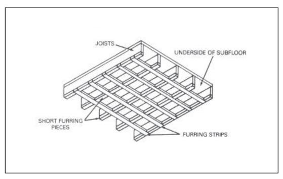
Figure 9-11. Furring strips on ceiling joists
