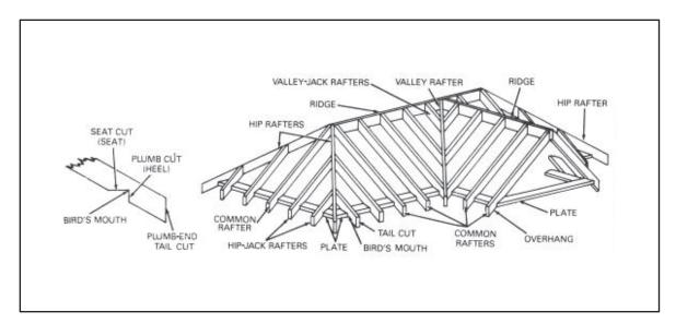
Figure 7-3. Common roof-framing terms
