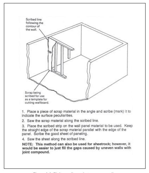
Figure 9-2. Fitting wall panels to uneven walls
