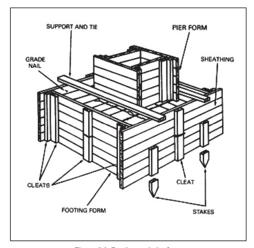
Figure 5-3. Footing and pier form
