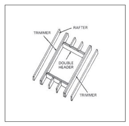
Figure 7-22. Roof-opening construction
