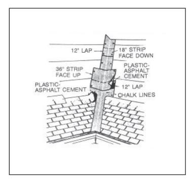
Figure 7-28. Open-valley flashing details using roll roofing
