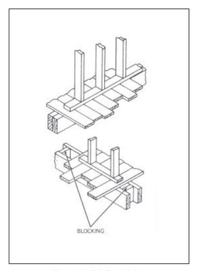
Figure 6-19. Reinforced joists
