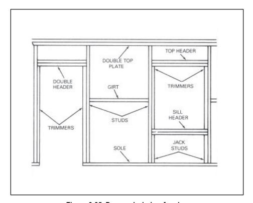
Figure 6-35. Door and window framing
