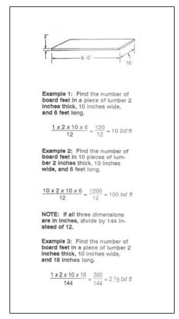
Figure 2-3. Examples of board-feet computations
