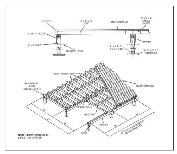
Figure 3-1. 20- x 40-foot TO building substructure
