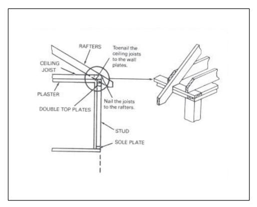
Figure 6-45. Built-up plate supporting joist and roof rafters
