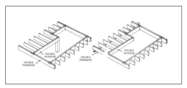
Figure 6-24. Double headers and trimmers
