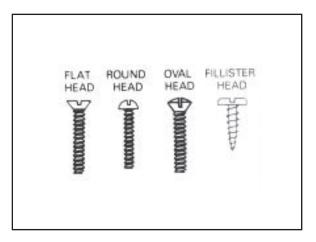
Figure 2-10. Sheet-metal screws
