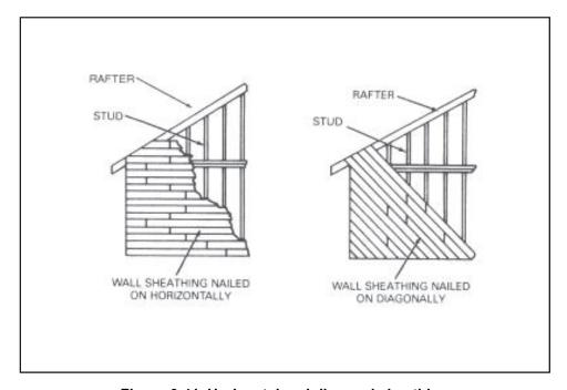
Figure 6-41. Horizontal and diagonal sheathing
