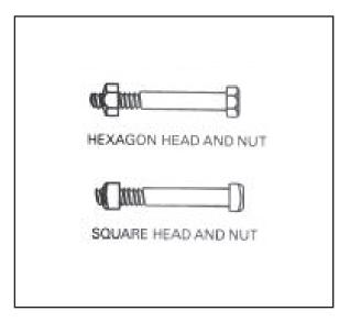
Figure 2-12. Machine bolts
