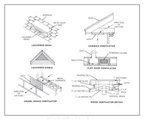
Figure 6-49. Types of ventilators
