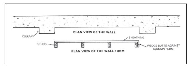
Figure 5-10. Wall form for curtain walls
