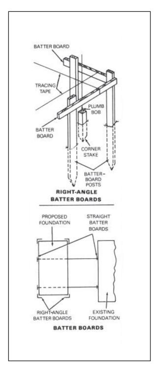
Figure 4-3. Locating batter boards
