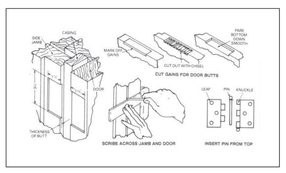
Figure 8-11. Installing door butts (hinges)
