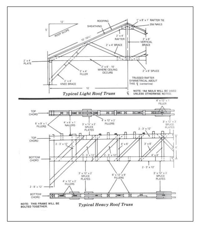
Figure 1-18. Roof trusses
