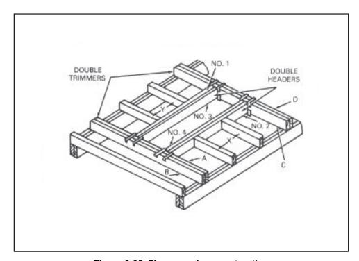
Figure 6-25. Floor-opening construction
