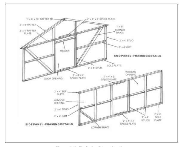
Figure 6-29. Typical wall construction
