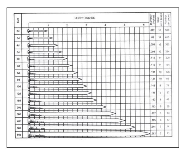
Figure 2-5. Sizes of cut nails
