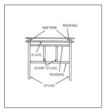
Figure 6-47. Framing for stovepipe
