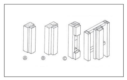
Figure 6-33. T-Post construction
