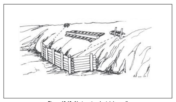
Figure 10-10. Abutment and retaining wall
