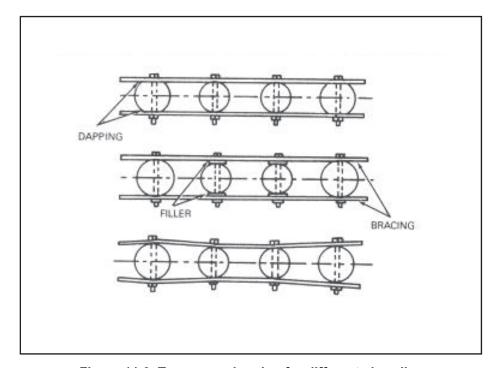
Figure 11-9. Transverse bracing for different size piles
