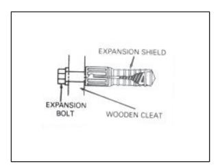
Figure 2-14. Expansion bolt and shield
