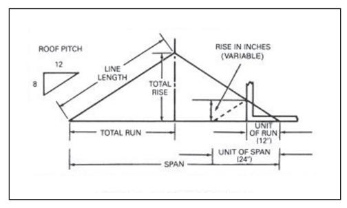
Figure 7-6. Determining roof pitch
