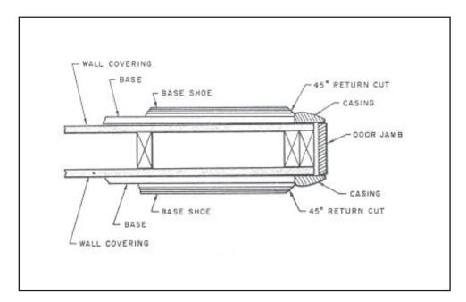
Figure 9-9. Base-shoe trimming
