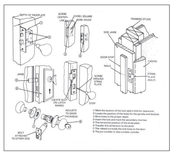
Figure 8-13. Installing lock and strike plate
