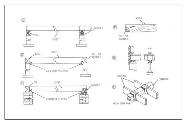
Figure 6-20. Sill and joist connections
