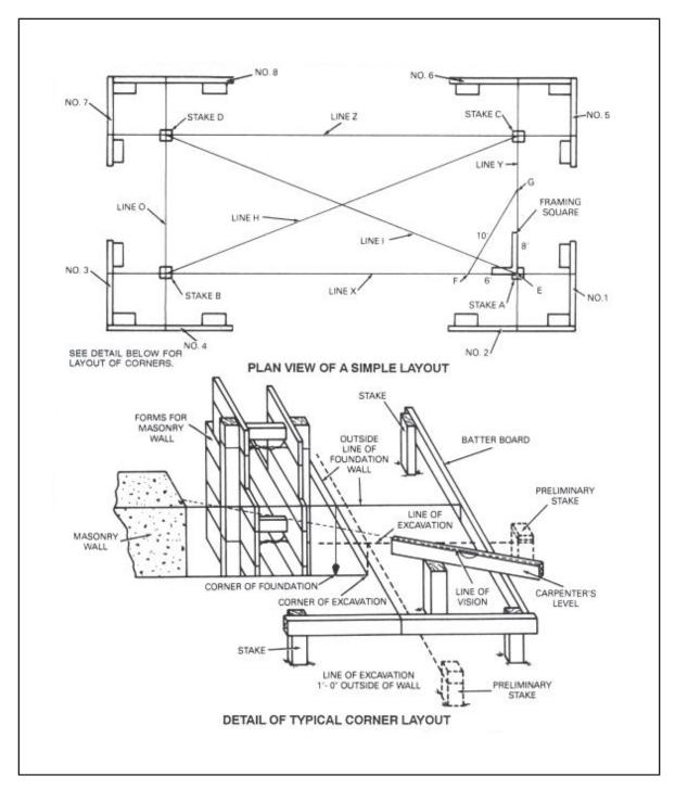
Figure 4-4. Laying out building lines from batter boards
