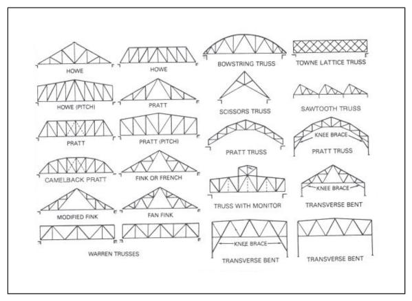
Figure 7-12. Types of trusses
