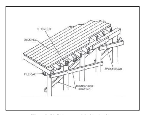
Figure 11-10. Stringers and decking in place
