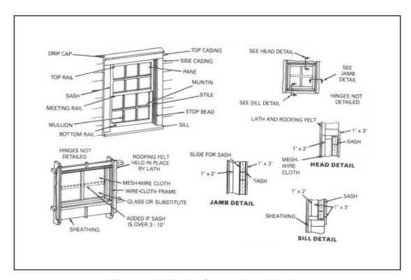
Figure 8-15. Window frame and sash details
