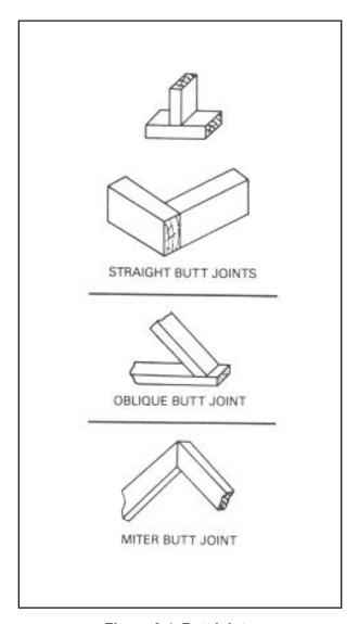
Figure 6-4. Butt joints
