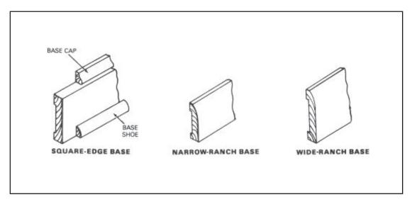
Figure 9-6. Types of base molding
