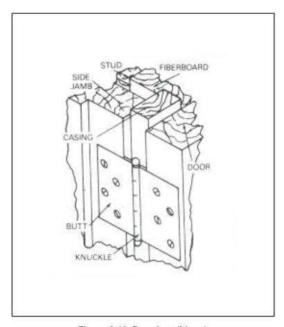
Figure 8-10. Door butt (hinge)
