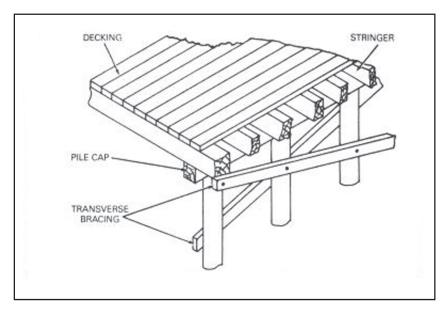
Figure 11-8. Capping and bracing piles
