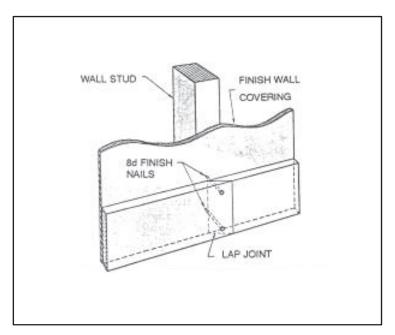
Figure 9-8. Trim lap-miter joint
