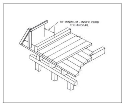
Figure 10-17. Solid-plank deck
