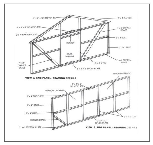
Figure 1-15. Typical wall-panel framing details
