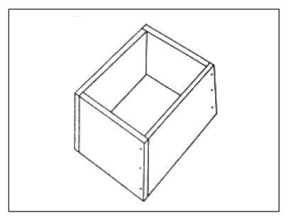
Figure 5-2. Typical small footing form
