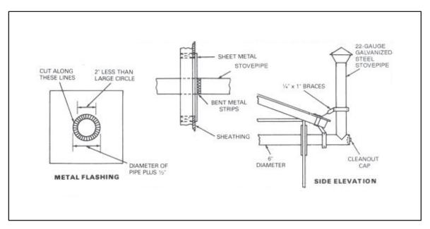
Figure 6-48. Installing stovepipe
