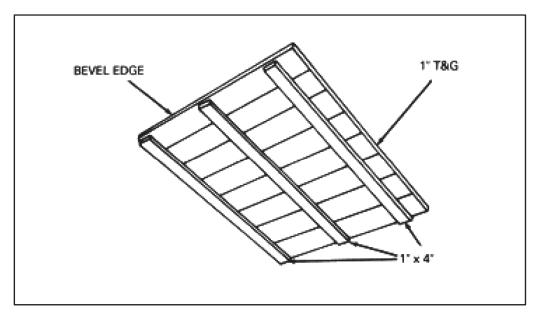
Figure 5-14. Floor slab form
