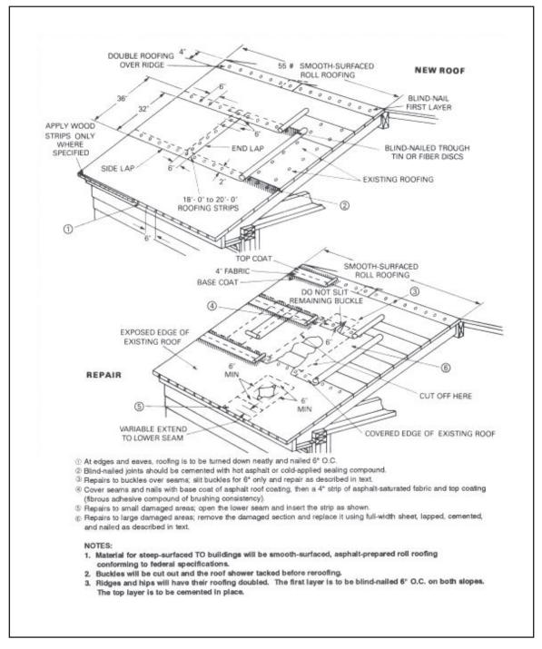
Figure 7-33. Smooth-surfaced roll roofing
