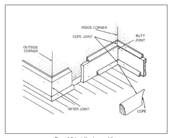
Figure 9-7. Installing base molding
