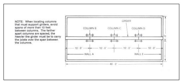
Figure 6-16. Column spacing
