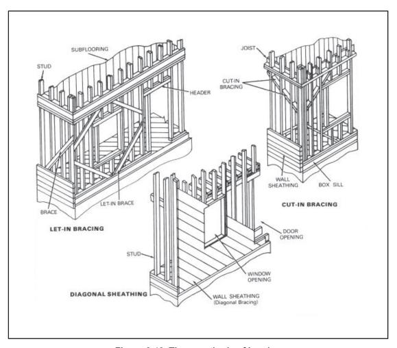
Figure 6-40. Three methods of bracing
