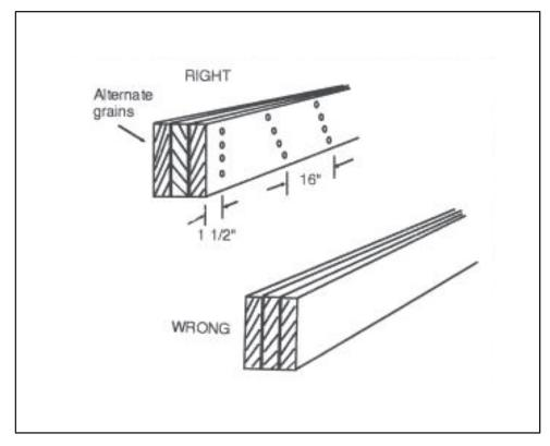
Figure 6-13. Built-up girder lumber arrangement
