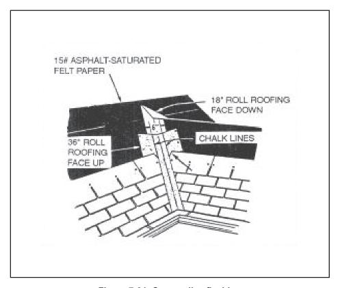
Figure 7-31. Open-valley flashing
