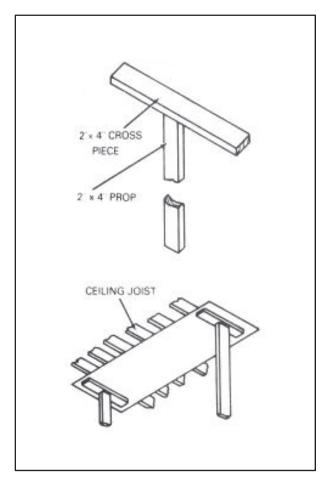
Figure 9-10. Brace for holding ceiling panels
