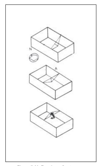
Figure 7-20. Erecting rafter trusses
