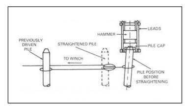
Figure 11-3. Realigning with a block and tackle
