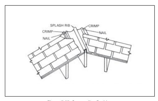
Figure 7-27. Open-valley flashing
