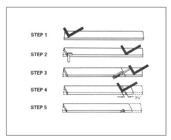
Figure 7-8. Scale or measurement method
