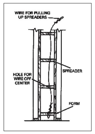
Figure 5-7. Removing wood spreaders
