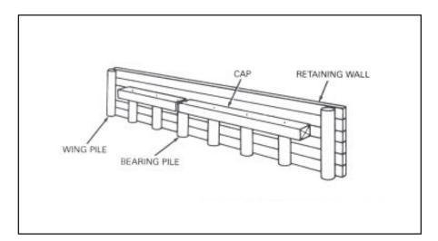
Figure 10-3. Pile abutment and retaining wall
