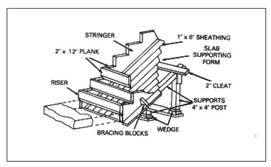
Figure 5-15. Stairway slab form
