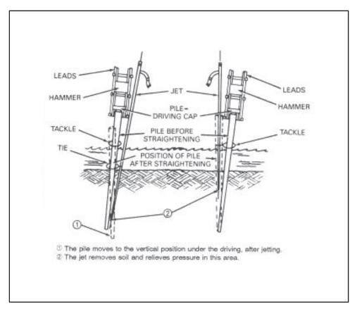
Figure 11-4. Realigning with a jet
