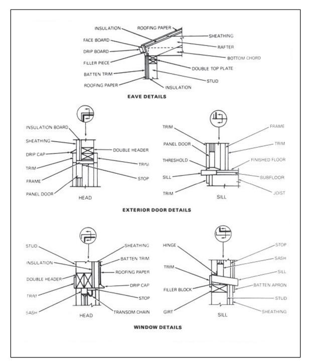
Figure 1-10. Typical eave, door, and window details
