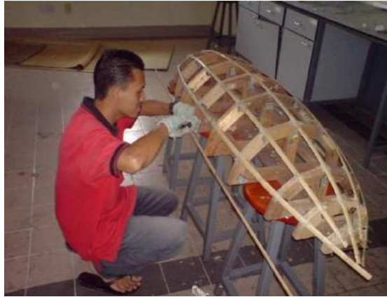
Figure 34-9 Attaching bamboo stick to the frame structure
