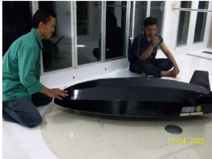
Figure 36-3 Installing the model in the test section
