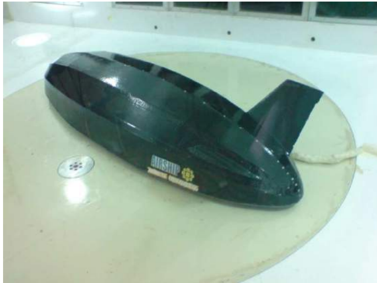
Figure 36-6 Pressure measurement testing at 25° angle of attack
