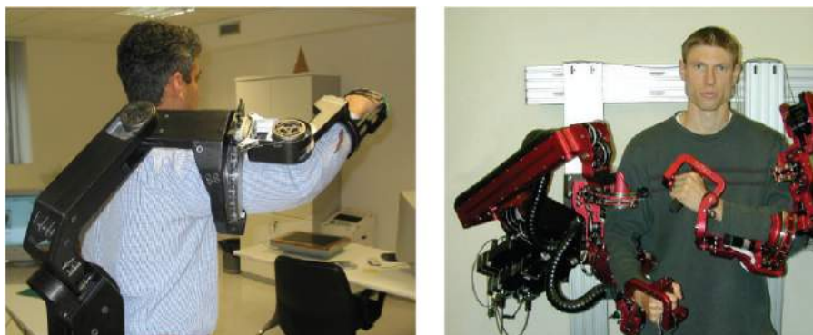
Figure 1.15: Exoskeletons designed by PERCRO (left) and the University of Washington (right) for medical rehabilitation.
