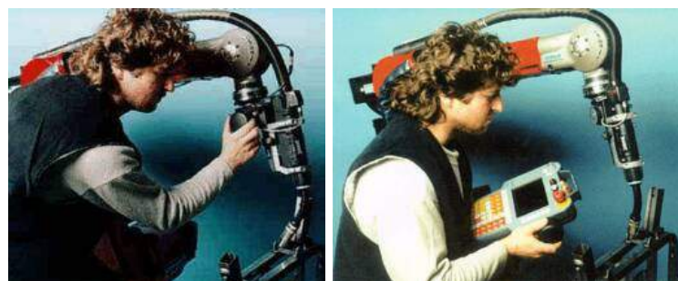
Figure 3.3: Programming by pasive guiding vs. programming by teach-pendant.
