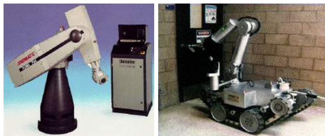
Figure 1.5: Samples of Industrial Robots: an old Puma 7000; HAZBOT II, a robot for handling explosives.
