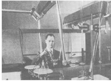
Figure 1.2: First teleoperated device. It was designed for radioactive material handling.
