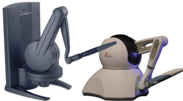
Figure 1.14: PHANToM haptic devices.
