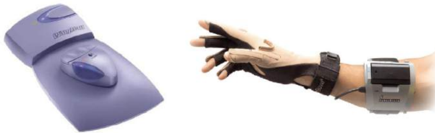
Figure 1.13: Two commercial haptic devices with tactile feedback through vibrations.
