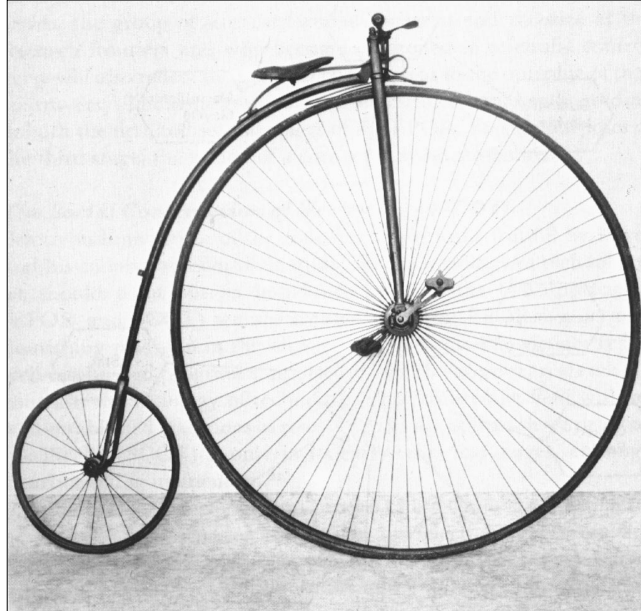
Figure 2.18: A typical Penny-farthing bicycle (Bayliss-Thomson Ordinary of 1878), a design for “young men of means and nerve”. The safety bicycle design (resembling the bicycle of today) evolved much later. Its rather bumpy development history was apparently strongly influenced by the social construction of “what a bicycle had to be”. Quotations from Pinch and Bijker (1987:28–34). Photograph courtesy of the Science Museum London/Science & Society Picture Library.
