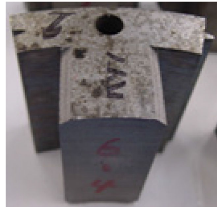
FIGURE 8 The trial manufactured stator core [Color figure can be viewed at wileyonlinelibrary.com ]
