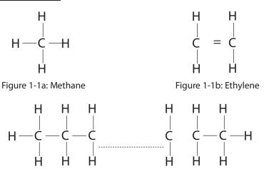
Figure 1-1c: Polyethylene Molecular Chain
