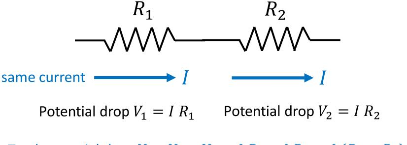
Total potential drop  $V = V_1 + V_2 = I R_1 + I R_2 = I (R_1 + R_2)$
