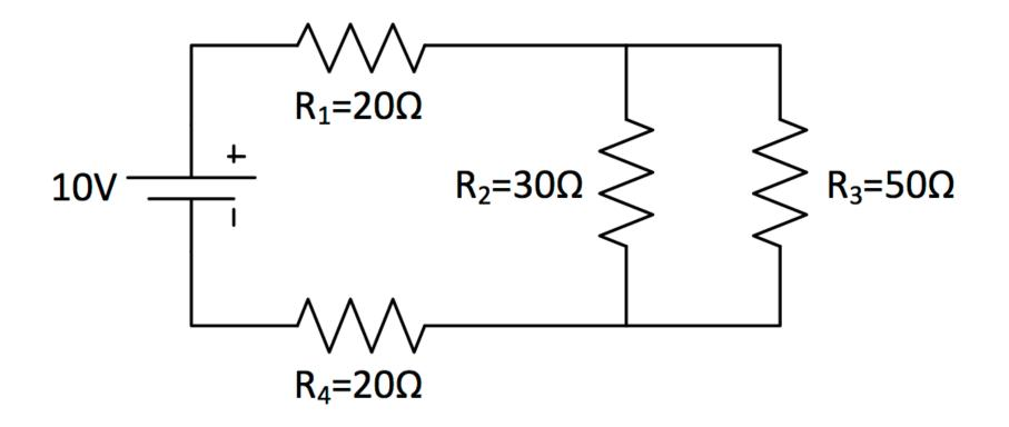
• When components are connected in series, the same electric current flows through them
