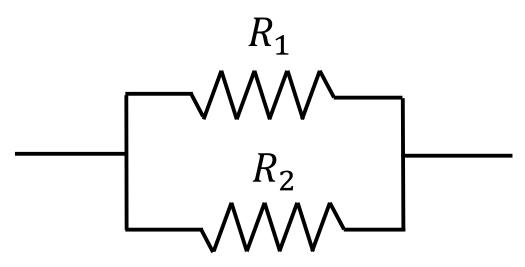
If two resistors are connected in parallel, what is the total resistance?
