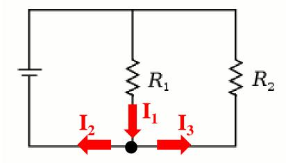
current in = current out  $I_1 = I_2 + I_3$   $I_3 = I_1 - I_2$  $I_3 = 2.5 - 4 = -1.5 A$
