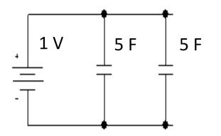
Potential difference across each capacitor = 1 VCharge on each capacitor  $Q = CV = 5 \times 1 = 5 C$
