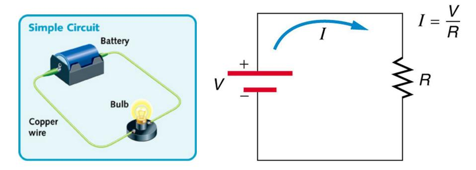
• R is the resistance (in Ohms  $\Omega$ ) to current flow
