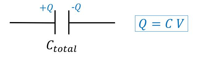
Total charge  $Q = C_{total}V = (C_1 + C_2)V$
