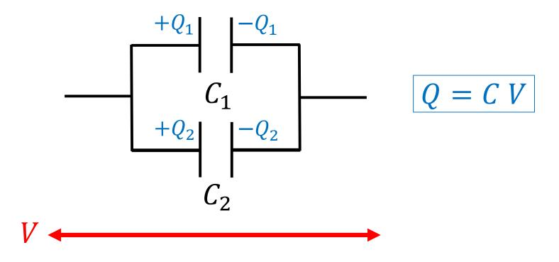
Total charge  $Q = Q_1 + Q_2 = C_1 V + C_2 V = (C_1 + C_2) V$
