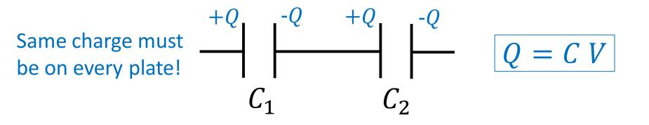
Potential drop  $V_1 = Q/C_1$  Potential drop  $V_2 = Q/C_2$
