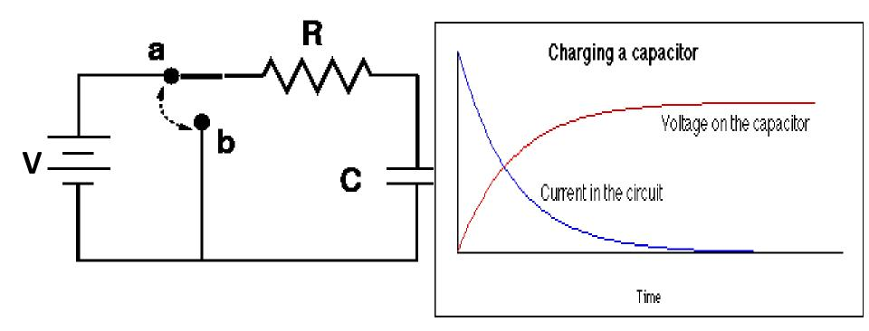
• When the battery is disconnected, the capacitor pushes charge around the circuit
