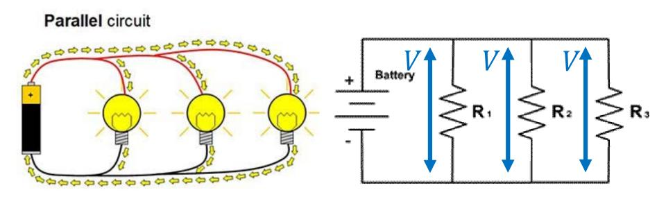
Points connected by a wire are at the same voltage!
