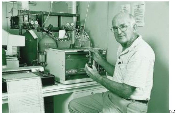
Figure 1 Barry McGlasson, University of Western Sydney Hawkesbury, Richmond Campus, at his gas chromatograph (fitted with flame ionisation detector) analysing ethylene concentration in gas samples taken from air exiting enclosed containers of harvested plums.
